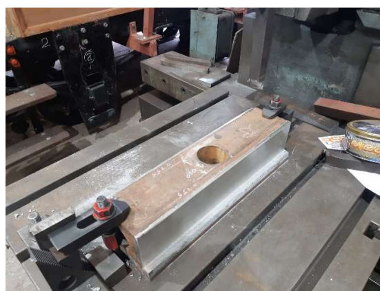
Crosshead slippers metallised and being machined
