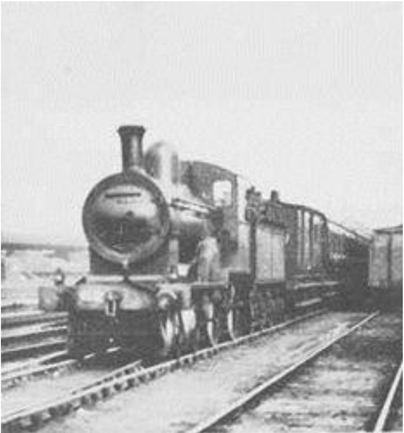
D14 No.62 on 3:15pm Waterford train leaving Kingsbridge on 20 th February 1940. This shows her with new frames, large cab and 60 class boiler with extended smokebox. (A. Donaldson)
