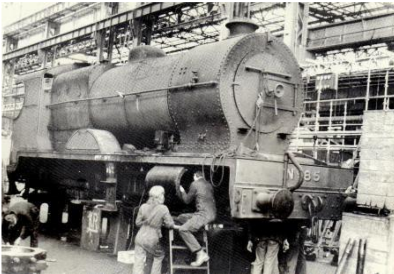
Dismantling No.85 in Harland's Engine Works - engine off its wheels, ashpan about to be dropped, apprentices measure the outside cylinders for wear, carbonisation, etc., while men behind buffer beam inspect the middle cylinder and slide valve faces. Eccentric straps are at bottom left of picture. (C.P. Friel)
