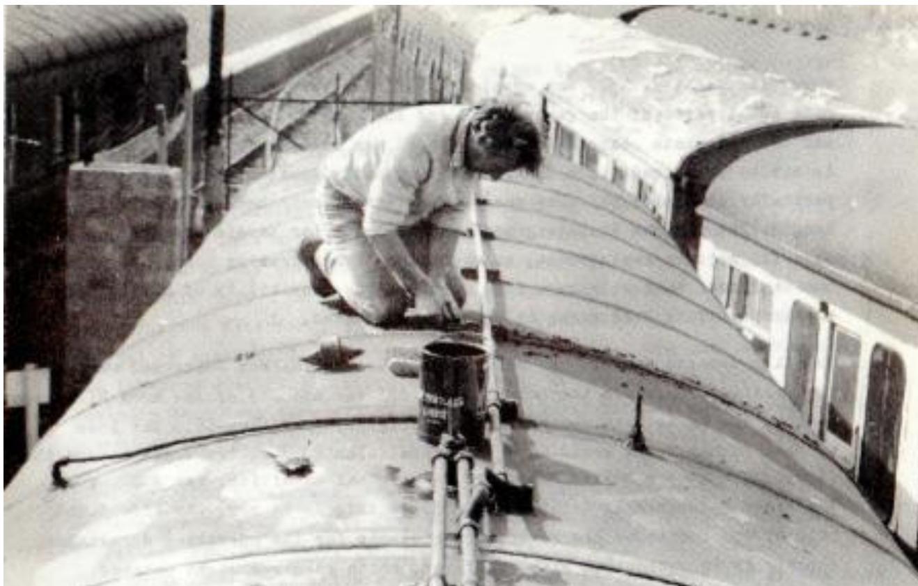
Carriageman at work - Ken Pullin sealing part of 1327's roof with bituminous paint at Whitehead. (C.P. Friel)
