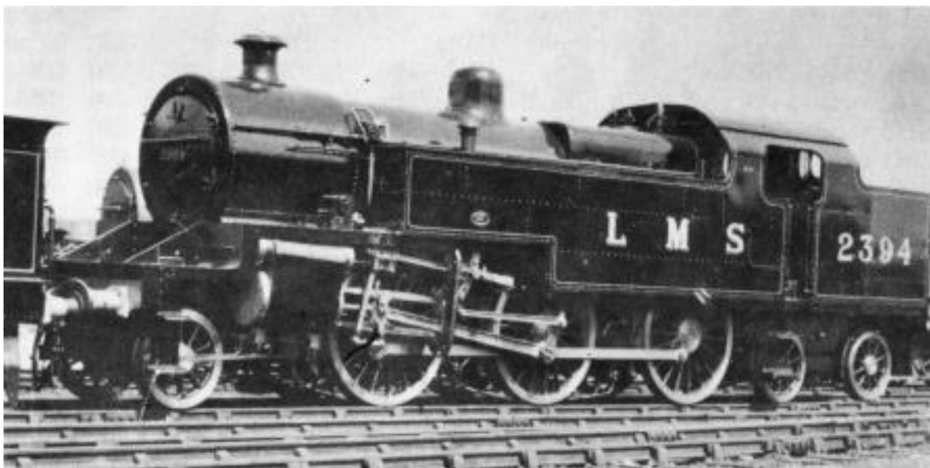
Original style Fowler 2-6-4T No.2394 in pristine condition at Derby. June 1933. (H.C. Casserley)
