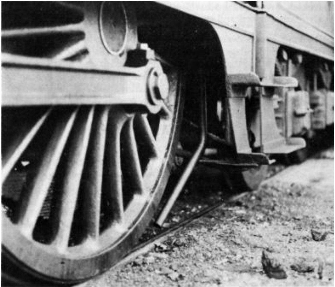
The hand-fed sand is deposited on the rail immediately to the rear of the rear-most driving wheels. (C.P. Friel)
