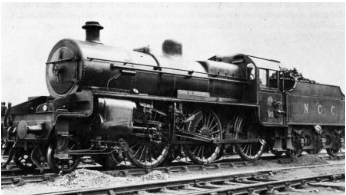
The derivation of the NCC Moguls from the original Fowler design can be clearly seen in this 1937 photograph of 90, but note the top feed and the styling of the cab. (Loco And General, No.6724)
