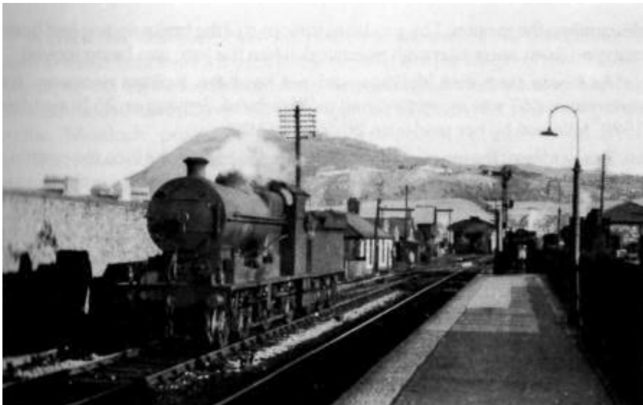
No.461, with CIÉ 'N' boiler, at Bray on 13 th August 1956. Several differences can be noted on the boiler, smokebox and tender. (H.B. Priestley)
