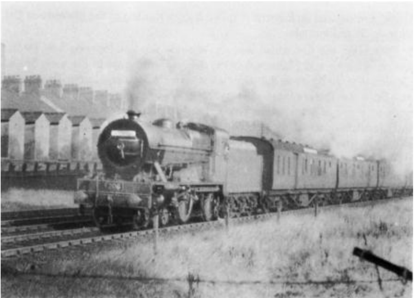
A year later, same train, same location but this time with VS No.206 "Liffey". The locomotive at this stage had not been fitted with the smoke deflectors which later became unique to this class. (A. Donaldson)
