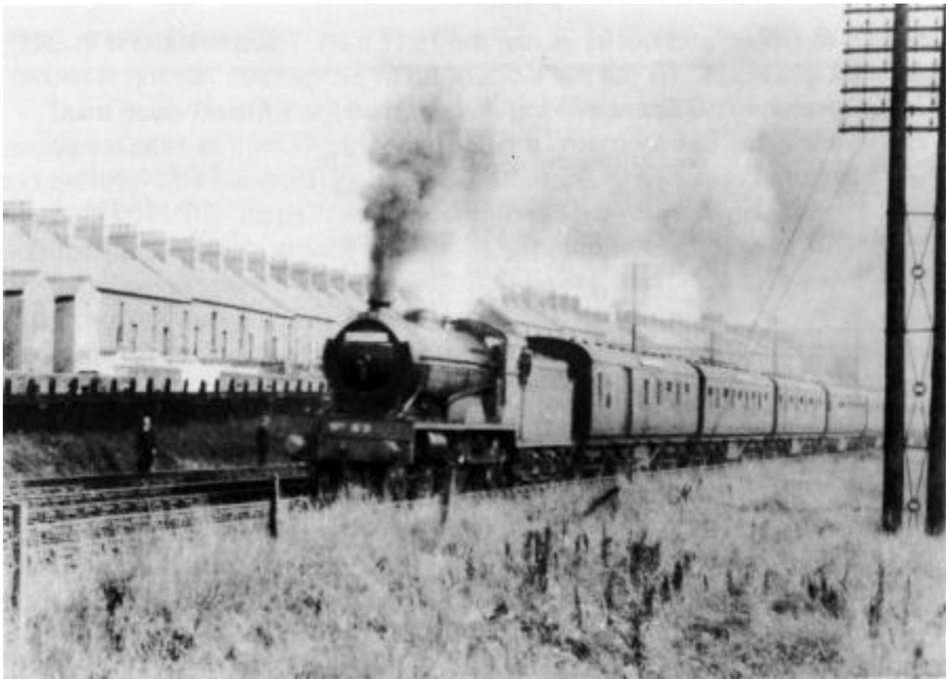
Compound No.83 “Eagle” between Central Junction and Adelaide on a morning up Enterprise in the summer of 1948. Note original round-topped firebox. (A. Donaldson)
