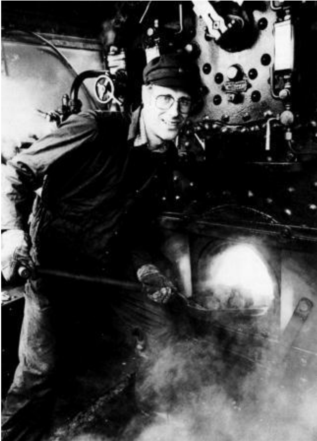
On one of No.461's early outings Peter Scott does some firing as a change from fixing. The strange pipe at the top left is part of a manometer temporarily fitted to measure smokebox vacuum when the locomotive was showing a reluctance to steam. (Belfast Telegraph)
