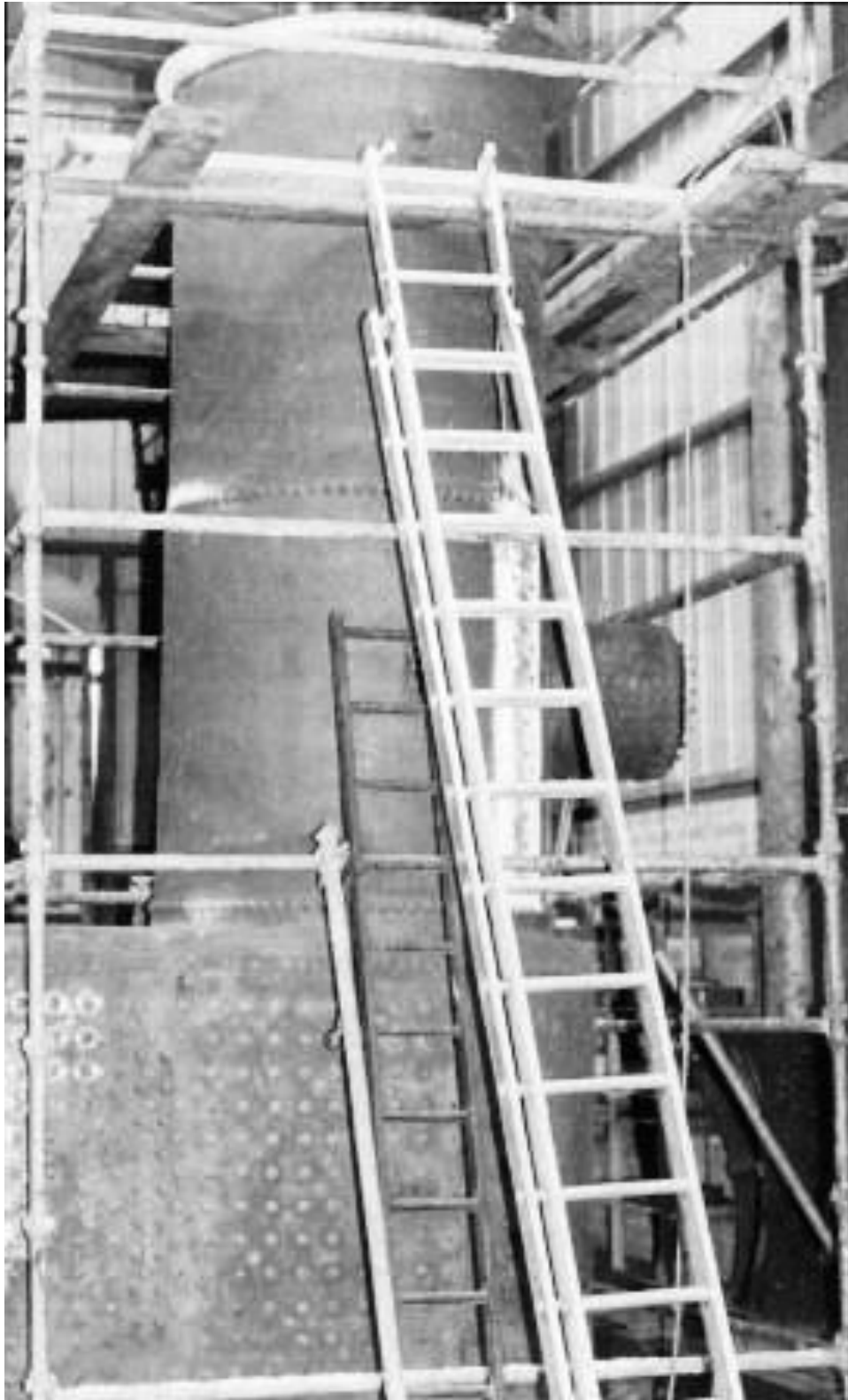
Super-gun or Easter Island statue? The boiler of No.186 positioned for welding of the front tubeplate and work on the firebox. It has since assumed a horizontal position. (I.C. Pryce)
