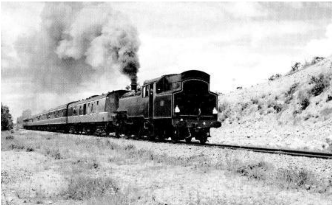
Contrary to the view held in certain quarters, these 2-6-4 tank engines were designed to run as fast backwards as forwards - and did so during their lives in company service. Here No.4 performs vigorously near Clara on one of the Tullamore shuttle trains in June 2004. (W.T. Scott)
