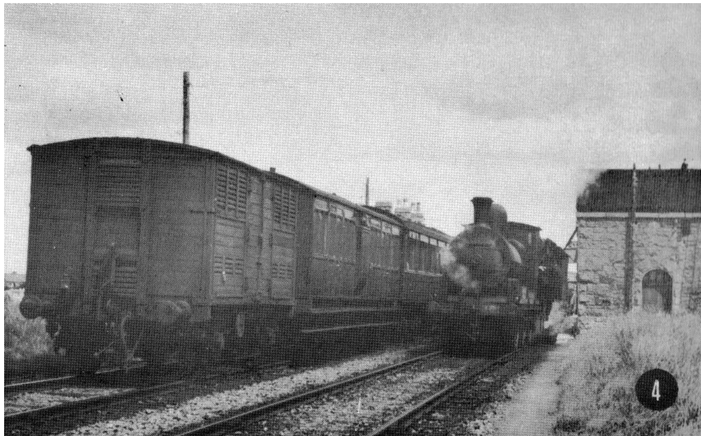
BALLYHAUNIS: J19 class 0-6-0 No.599 with No.3 (Lecarrow) ballast on 10 th July 1957. The ballast is seen here crossing an Up Westport train with a Midland van on the tail. The loco was Midland class L No.60 "Lough Owel" built by Broadstone in 1885. (D. Donaldson)
