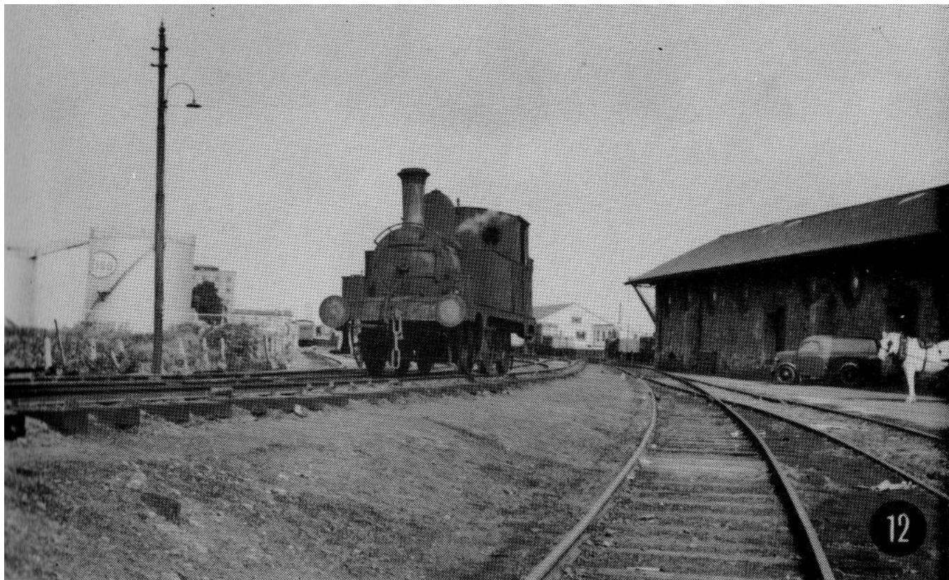
SLIGO: J26 class 0-6-0T No.558 in Sligo Quay goods yard on 22 nd August 1957. The loco was built in 1892 as Midland 113 "Gnat" by Kitson. (D. Donaldson)
