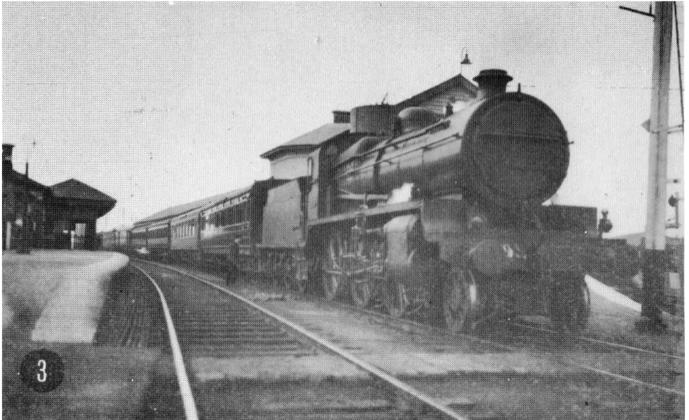
MULLINGAR: K1a class 2-6-0 No.393 on the Up Galway Mail at Mullingar in 1932. Note the Pullman Diner, second vehicle in the train. The loco, built from a kit of parts at Inchicore in 1930, was one of the second series of Woolwich Moguls with 6', as opposed to 5'6", driving wheels. (Kelland Collection, 48)
