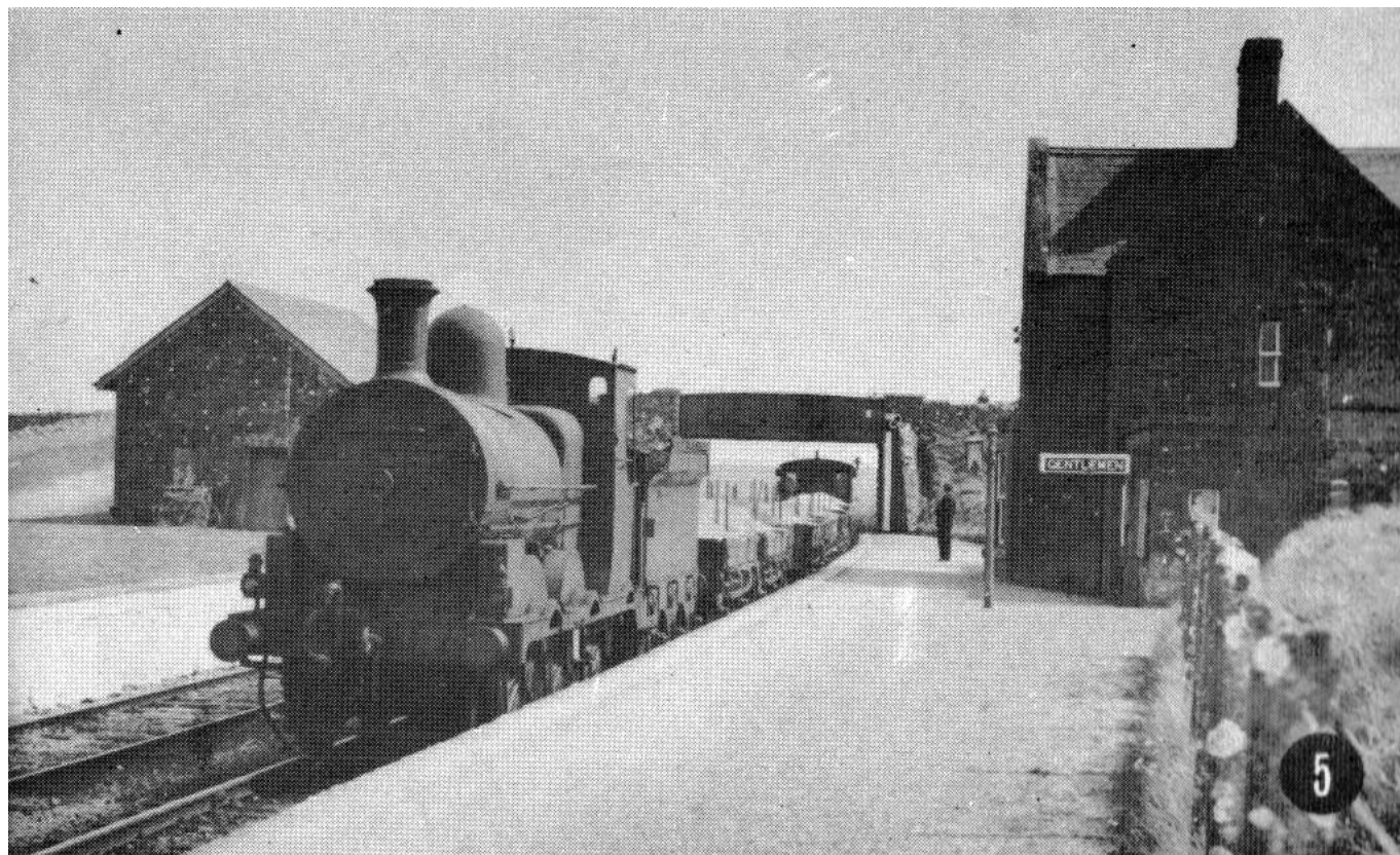
DONAMON: J19 class 0-6-0 No.597 with the Lecarrow ballast train on 19 th April 1957. The loco was Midland L class No.58 "Lough "Gill" built by Broadstone in 1885. (D. Donaldson)
