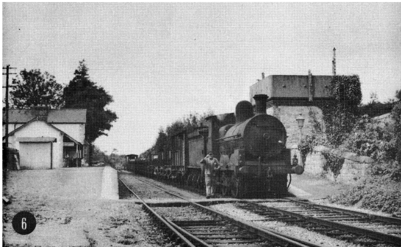
COLLOONEY (GS&WR): J19 class 0-6-0 No.599 again with the Lecarrow ballast at the northernmost station on the Burma Road, bound for Sligo on 22 nd August 1957. The loco is coupled to a 3,000 gallon tender off a larger scrapped loco. The point in the foreground leads to the Sligo Leitrim. (D. Donaldson)
