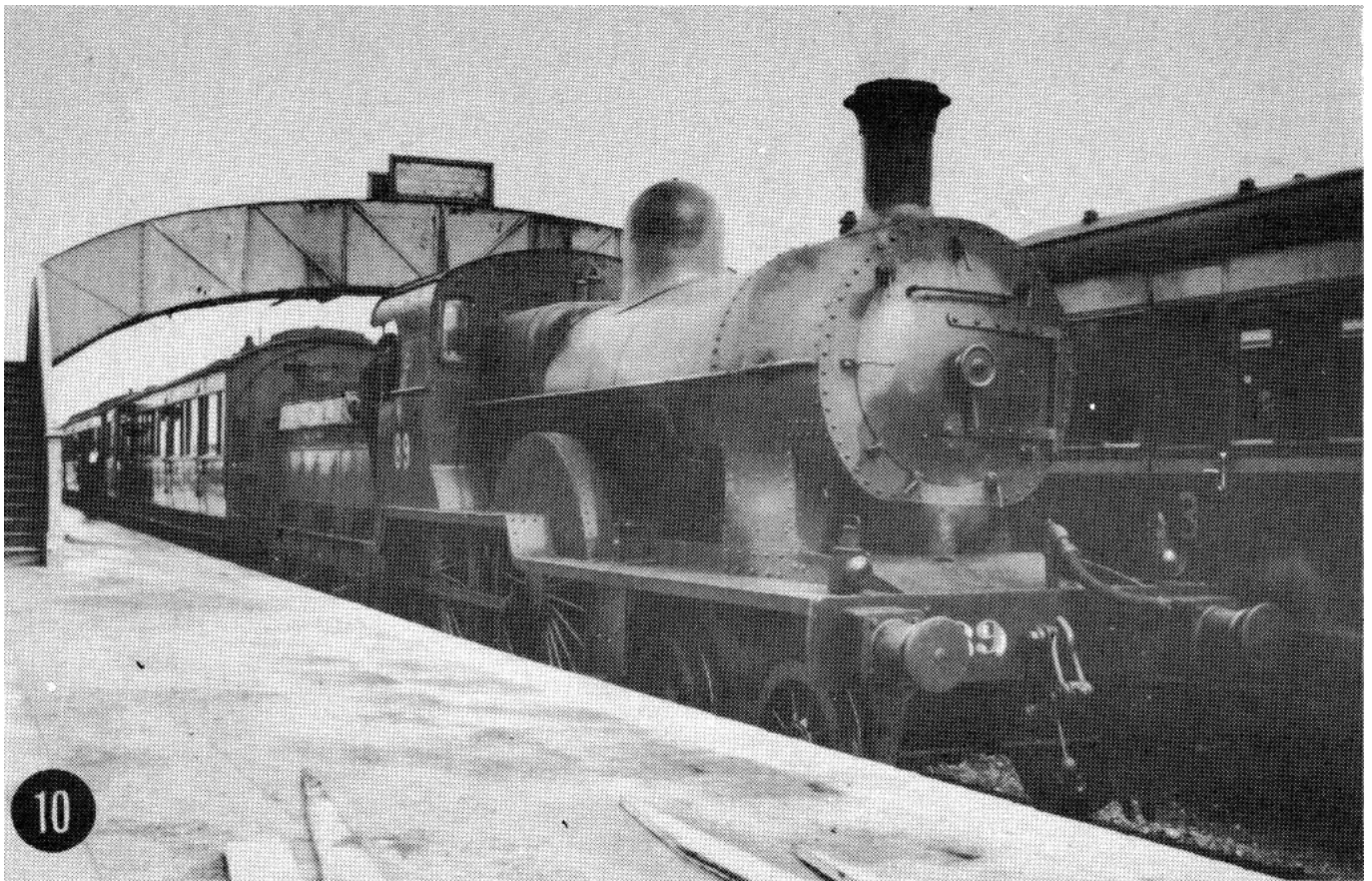
CLAREMORRIS: D14 class 4-4-0 No.89 (Inchicore 1886) with the 3:35pm Limerick to Sligo on 16 th April 1952 when the engine wasn't long out of the shops. The engine had been D13 class with a 700 class saturated boiler but here carries a Z class superheated boiler and is coupled to a 1,864 gallon tender. (R.M. Arnold)
