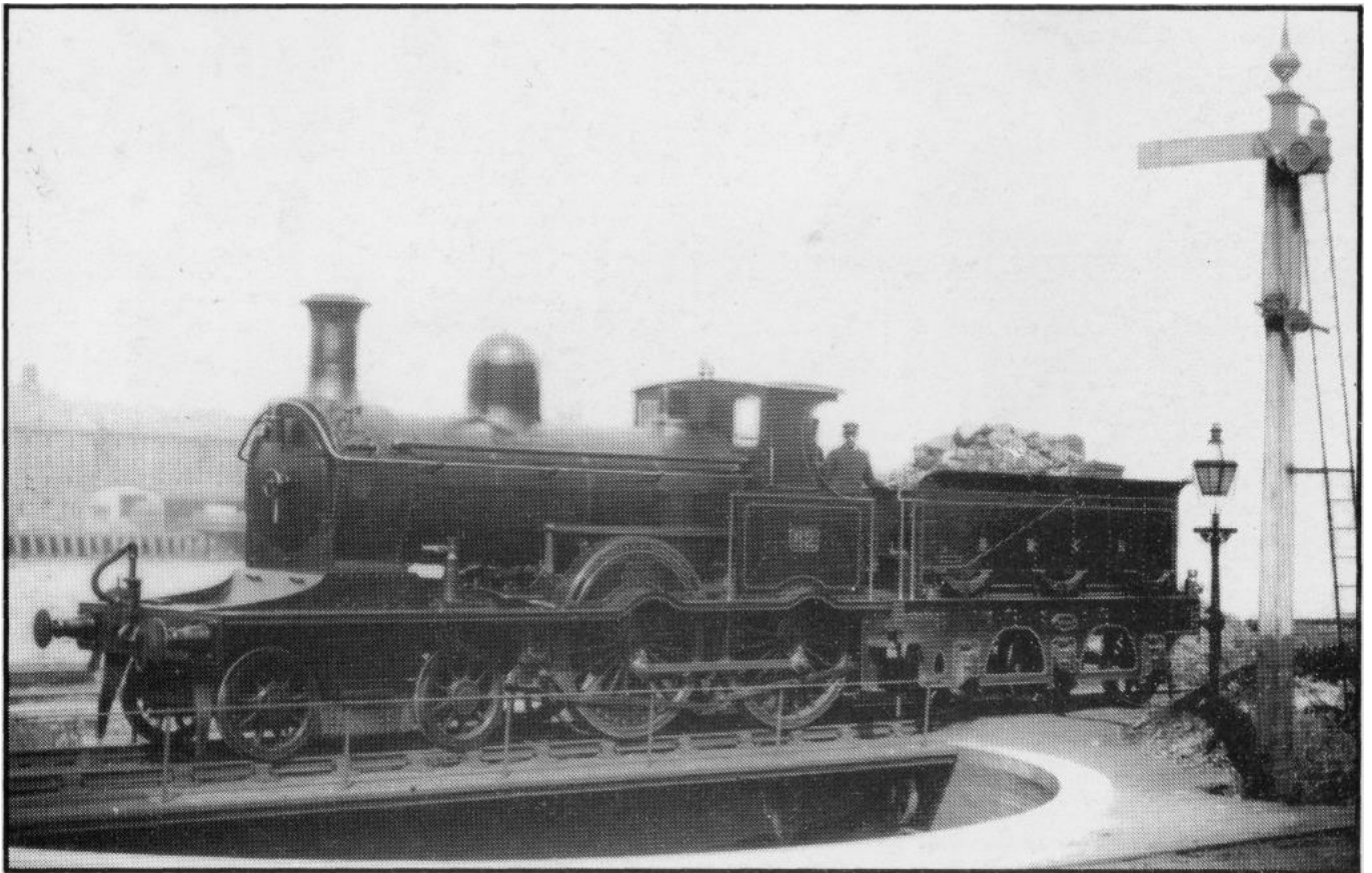
4-4-0 No.62, in BNCR days, on the old turntable at Waterside. This table was located on the river bank, and was protected by special signalling, as locomotives tended to foul the running lines when being turned. It was too short to turn a Mogul, and was therefore replaced by the present turntable, which was originally at Cookstown Junction. (Loco and General Railway Photographs, 5918)
