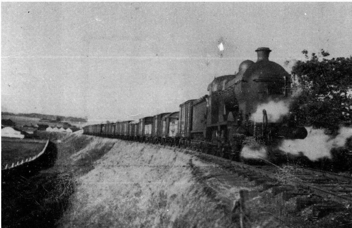
One of the 1935 batch of J5 class 0-6-0s (without the oiling crescent in the valancing) climbs away from Sligo Quay with a goods for Dublin North Wall. The date is 1935 and the banking engine is just visible on the tail. (Locomotive Publishing Company, 87328)
