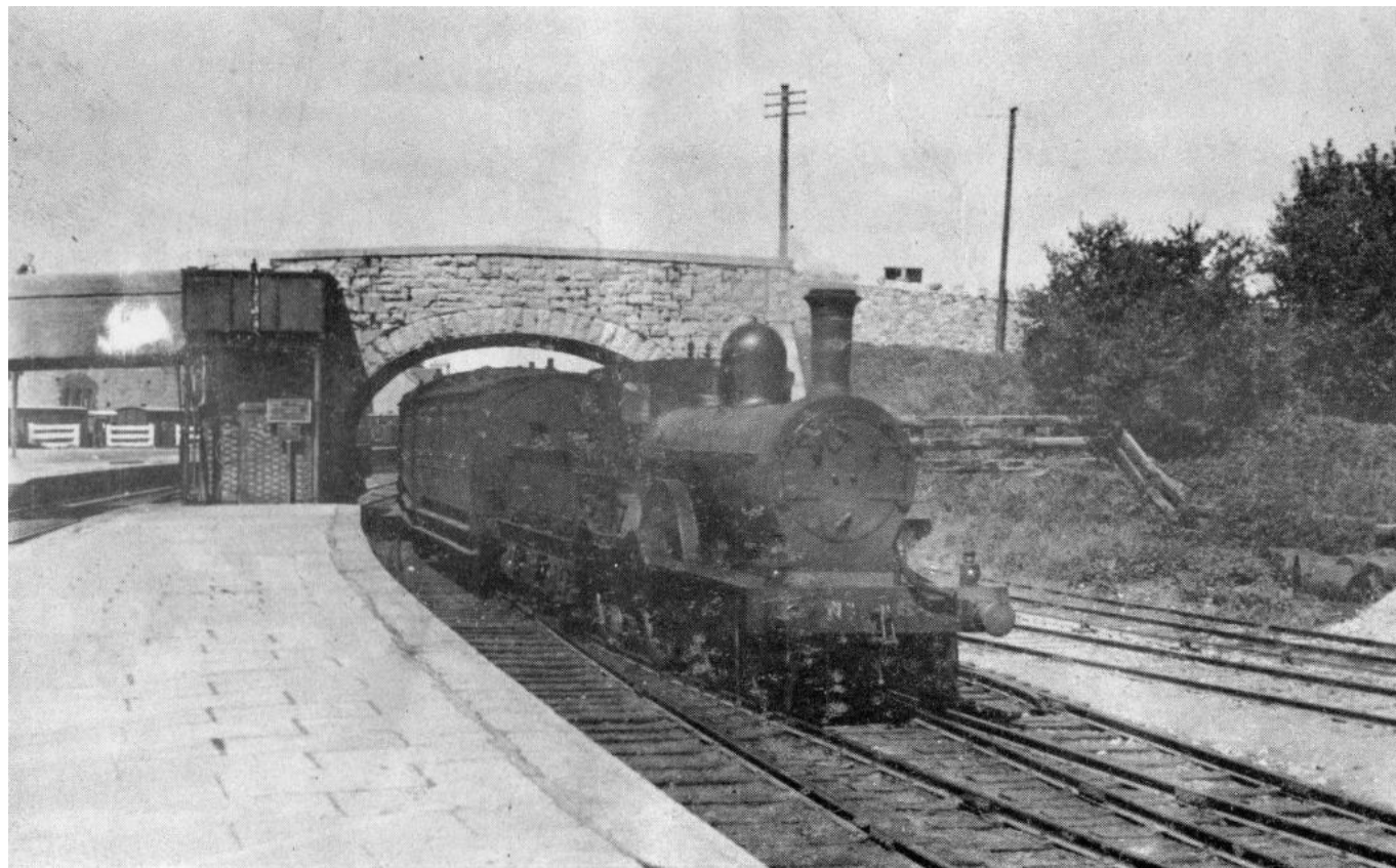
One of the famed 60 Class (D14), No.64 swings under the bridge at the north end of Ennis with a train from Sligo in the late 1920s. The loco is here fitted with a double-door smokebox but this had been altered before the photo below was taken. (Photographer unknown)
