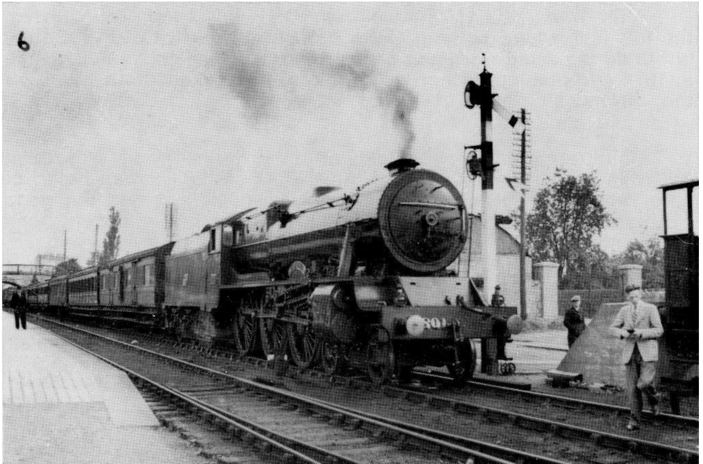
B1A class 4-6-0 801 "Macha" pauses at Thurles with an Amiens Street to Cork IRRS special in 1949. The smokebox door has been disfigured with the mountings for the Centenary headboard. (Kelland Collection, 23281)
