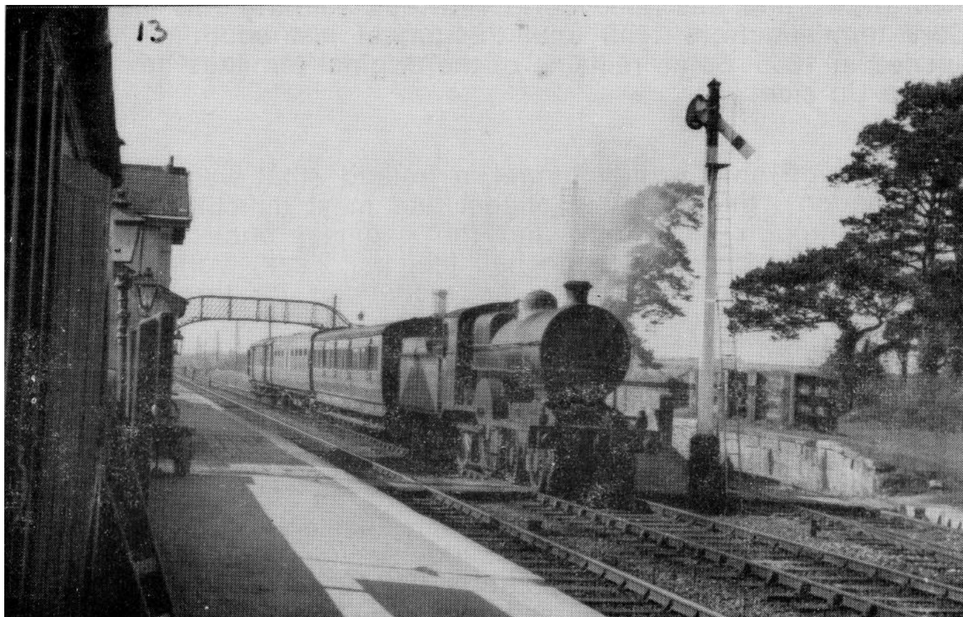
D2 class 4-4-0 332 passes Blarney with 7:15 a.m. Down Perishable on 13 th April 1955. This engine was rebuilt with superheater and piston valves in 1926 when the boiler was pitched 2¾ inches higher than her superheated sisters. She was later described as having a tendency to roll, making firing difficult and not a free steamer. (Drew Donaldson)
