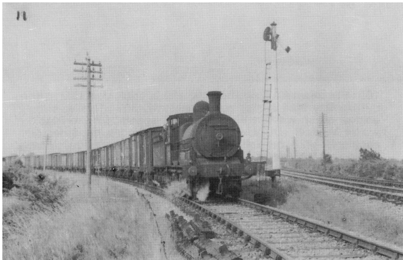
J15 class 0-6-0 164 is signalled off the Croom Branch at Rath Luirc Junction with 15:00 Limerick to Cork Cement special on 2 nd August 1957. The main line curves away towards the Junction behind the uncounterweighted, electrically-operated signal. (Drew Donaldson)
