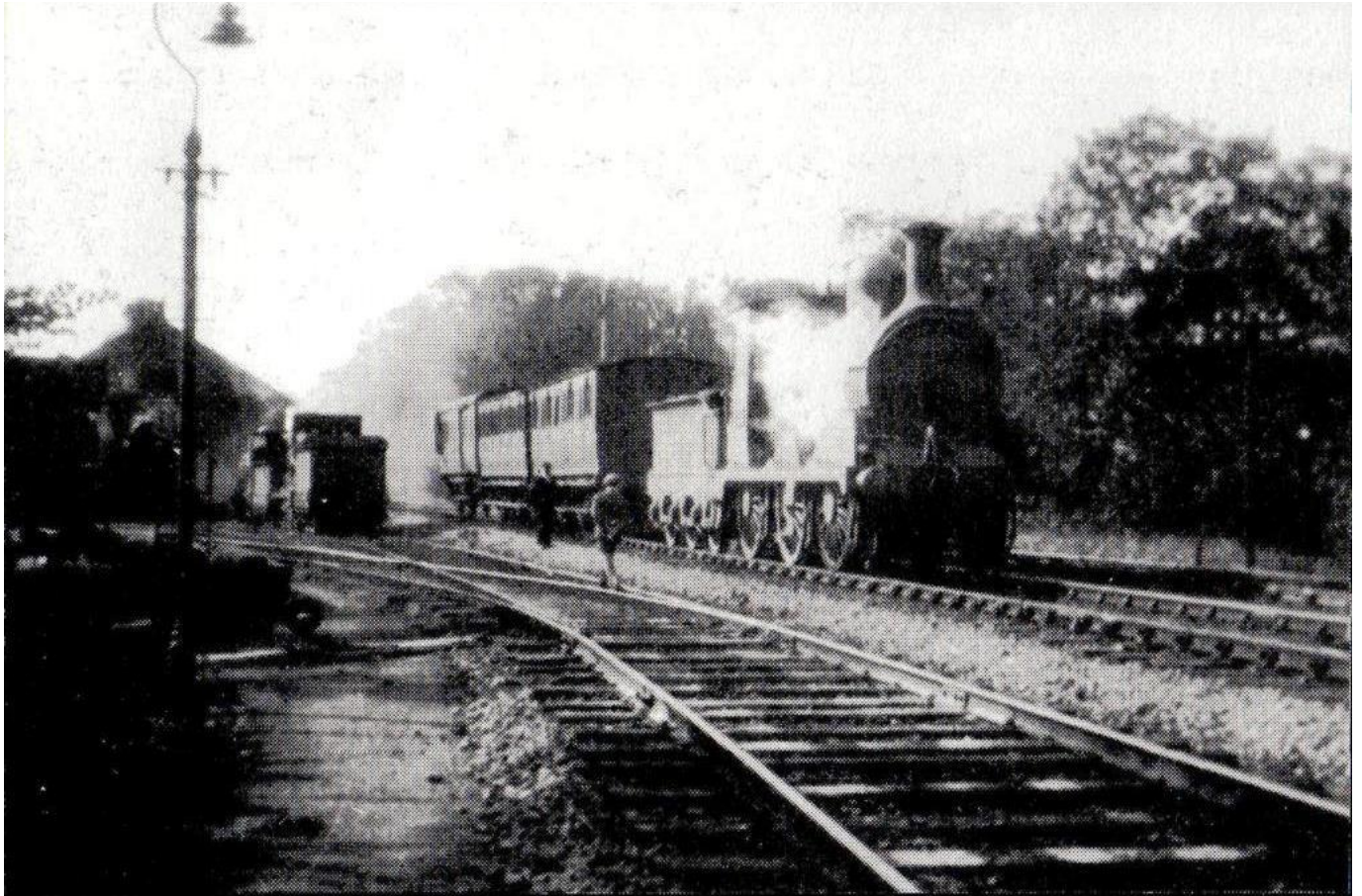
Sligo: No.607 Class J19 0-6-0. Built Broadstone 1889. The train is Clayton Car working the 10:50 ex Mullingar in September 1930. (R.N. Clements)
