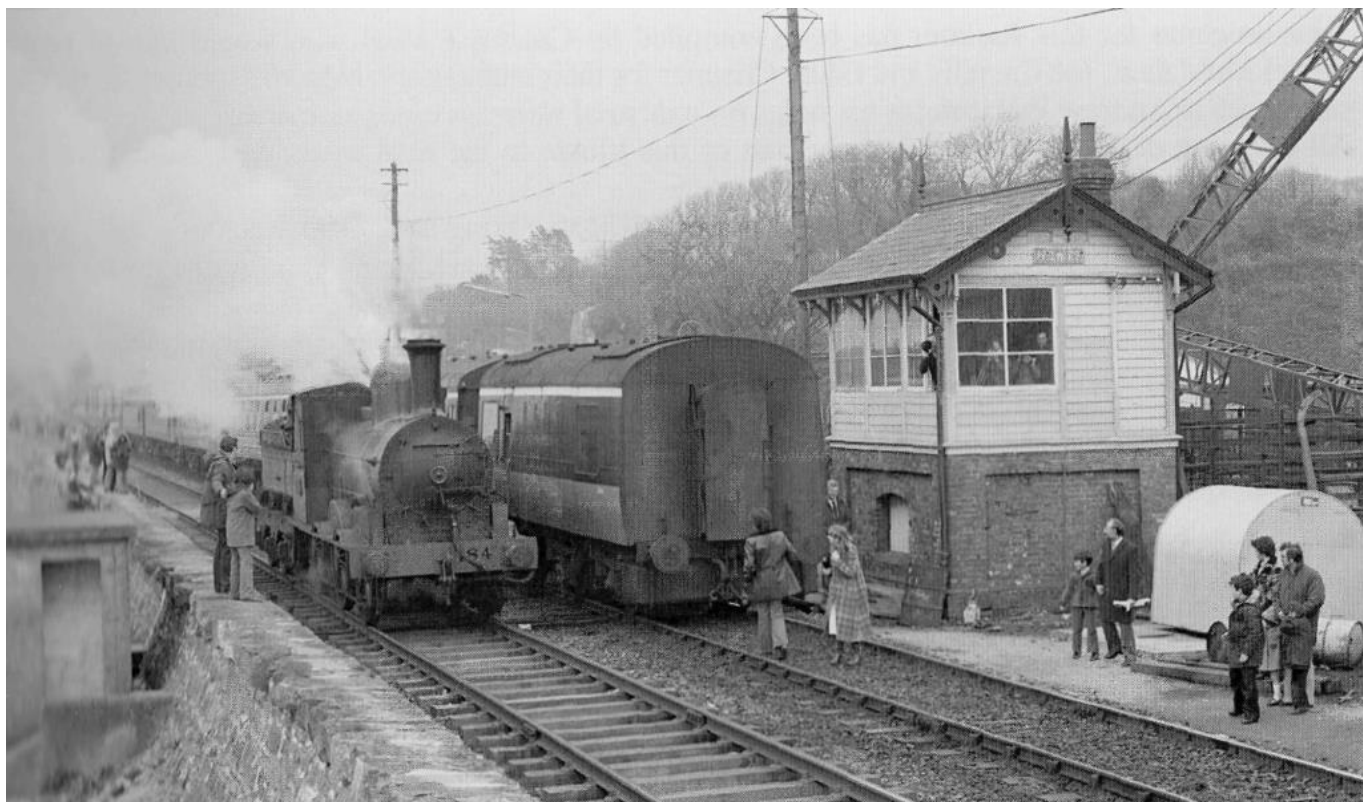
Howth: No.184 is seen running round the train on one of her visits here on Sunday 13 th April 1980. Note the signal cabin on the right and the casual approach to trespassing. Heating Van 3154 was one the last batch of 4-wheel HVs built at Inchicore in 1964. (Joe Cassells)
