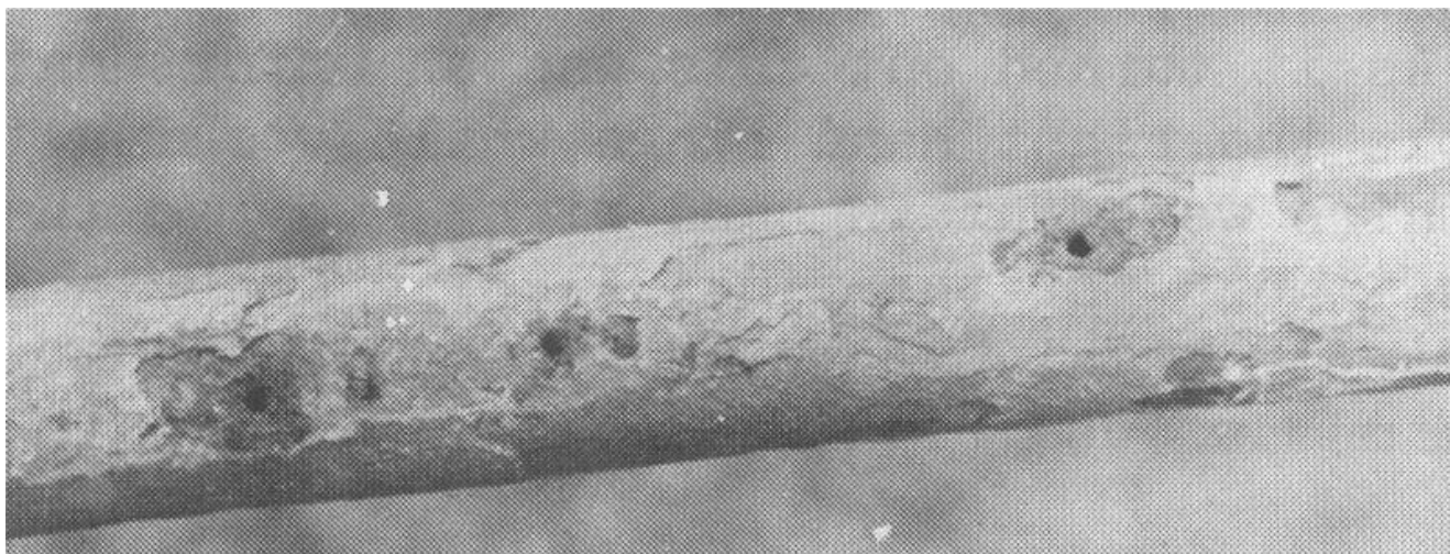
The tube which caused No.4's failure - showing scale coatings chipped away to show some of the holes. The hole on the right is approximately ¼ inch across. (C.P. Friel)
