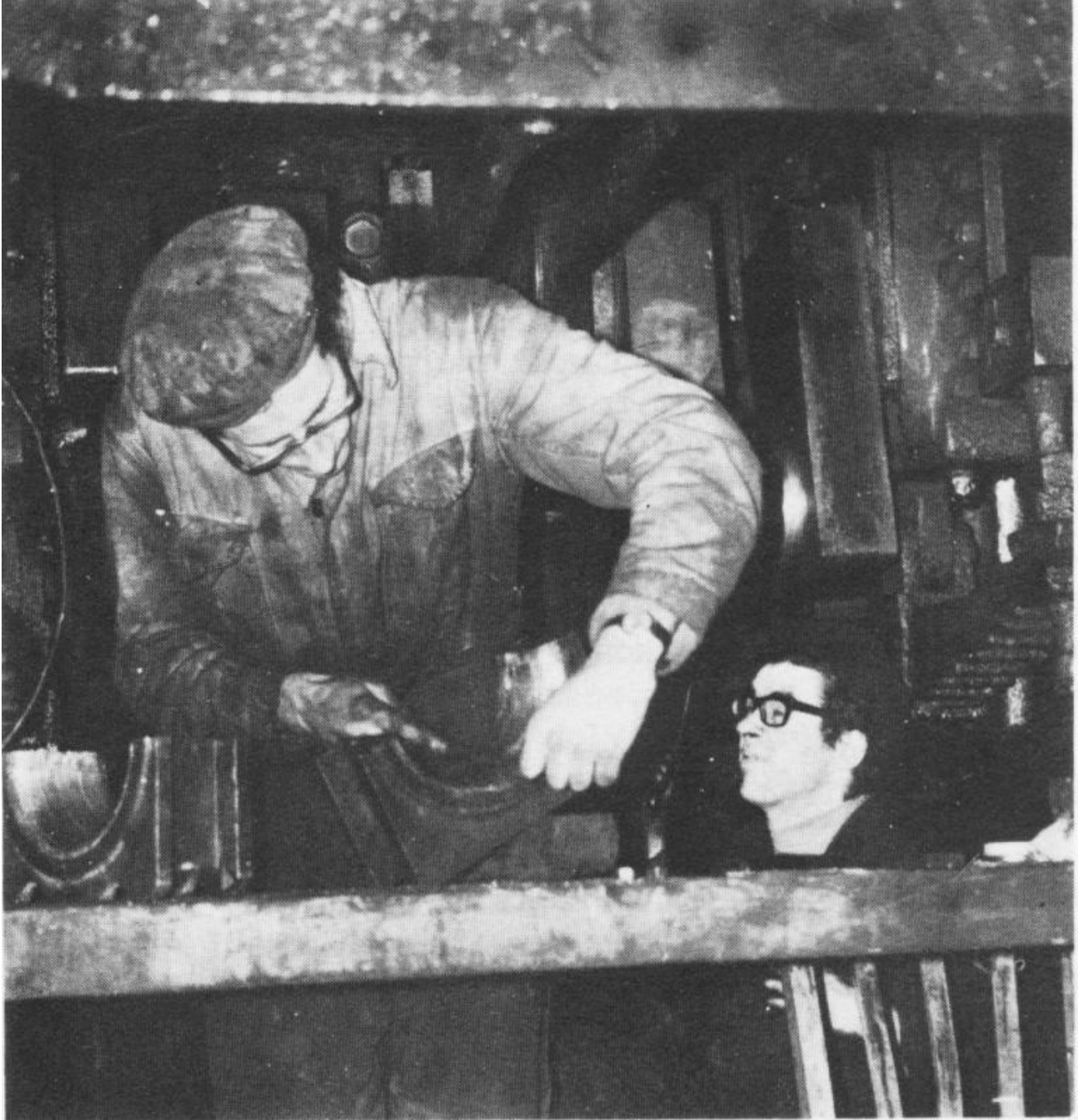
Peter Scott works at fitting No.186's left-hand big end bearings while John Friel (right) waits to help with the next lift. (C.P. Friel)
