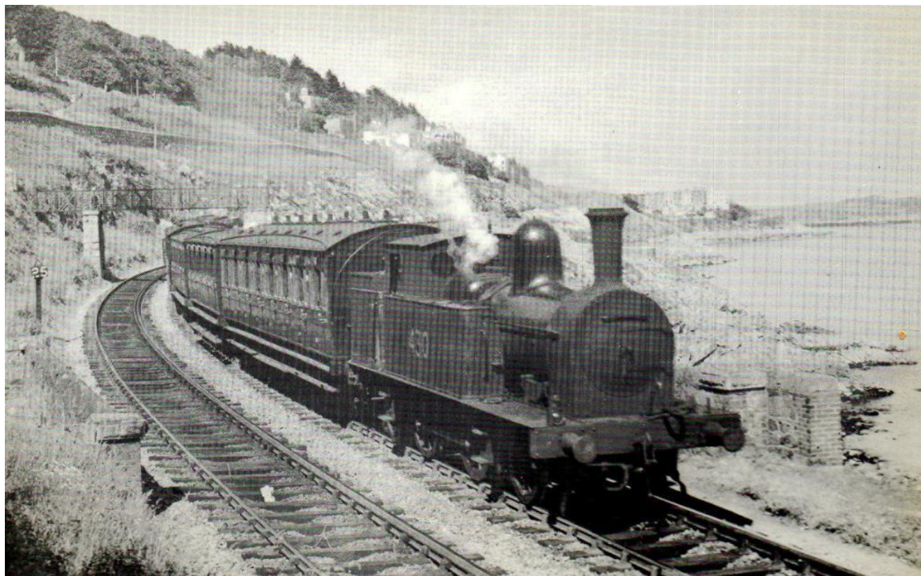
Great Southern F2 class 2-4-2T No.430 near Sandycove with a Dublin to Bray train in June 1951. Built as DSER No.11 at Grand Canal Street in 1886, this engine ran for a time on the Belfast and County Down. (Derek Cross)
