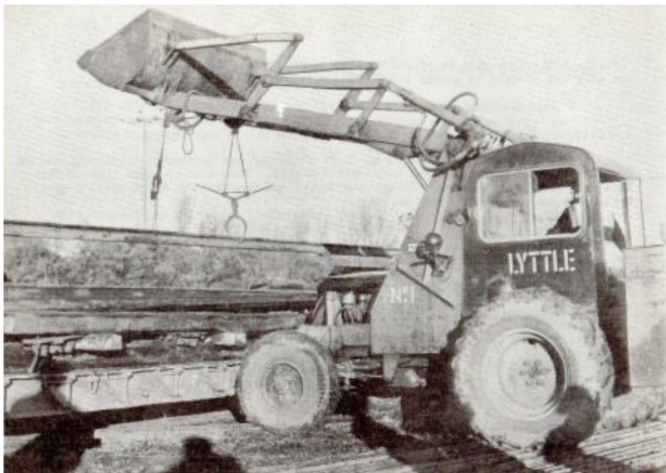
The work of removing trackwork from Greenisland was greatly facilitated by the work done by our loading shovel, seen here making light work of lifting a 60 foot rail onto the low loader using two track tongs suitably roped to the bucket. (C.P. Friel)
