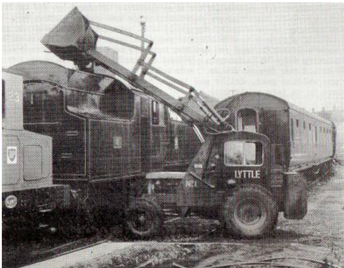
Coaling has long been a bane at Whitehead but now solved with the arrival of our loading shovel, seen here making light work of lifting something like half a ton of coal into No.4's high bunker. (C.P. Friel)
