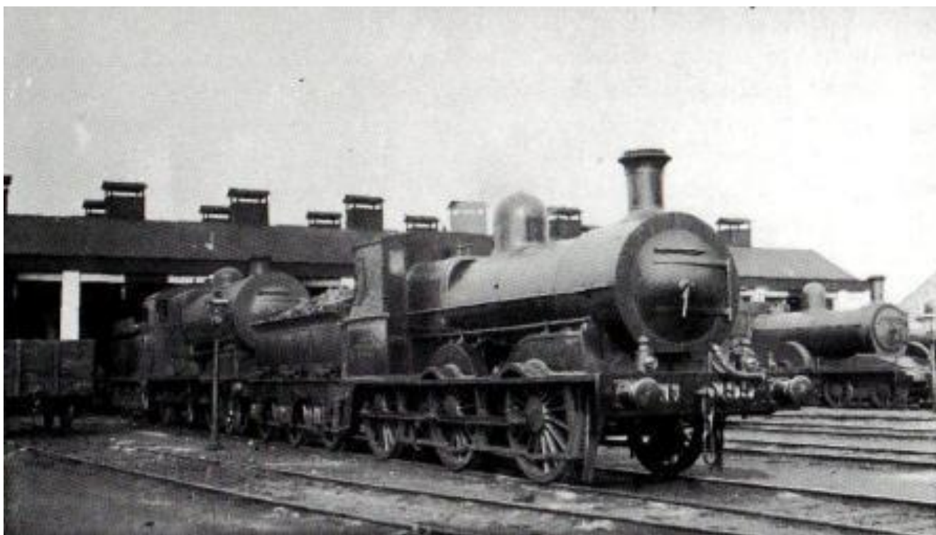
199 is seen here at Inchicore in 1932, shortly after receiving the superheated 'Z' boiler. The smokebox, with flush rivets, and devoid of dogs and a central hand wheel, is in total contrast to later practice. (Kelland Collection 23070)
