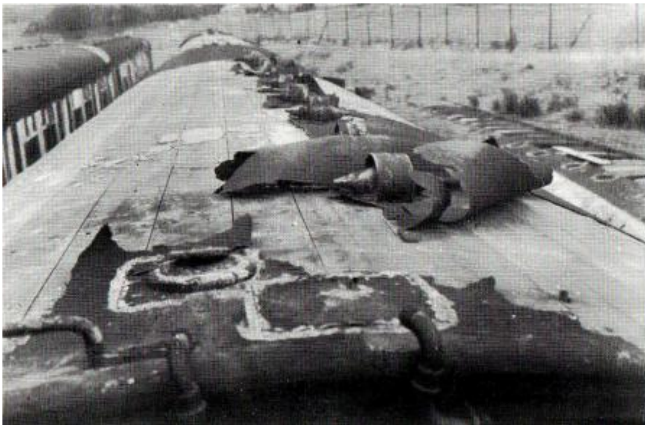
Carriageman's Nightmare. This shows the problem which we face with many of our carriages. The roof covering of this coach (342) has completely disintegrated, leaving the wooden planking of the roof (which is not watertight) exposed. (C.P. Friel)
