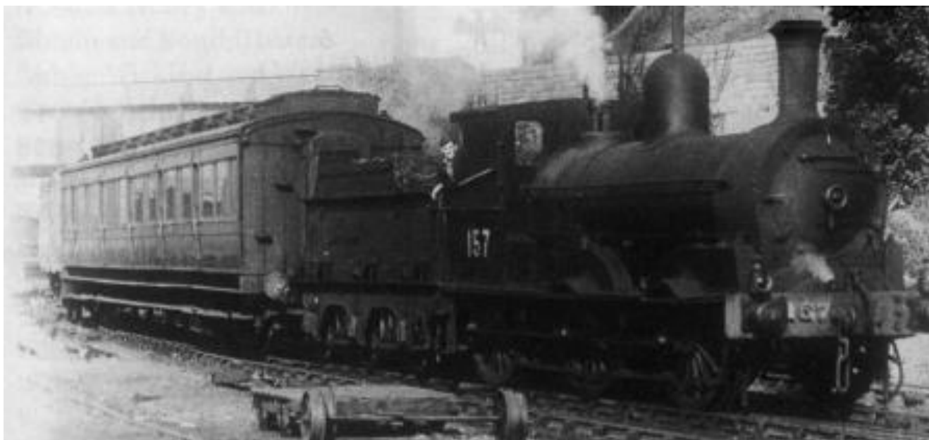
J15 No.157 with the 10am Waterford-Macmine Junction via New Ross. The carriage is an ex-GSWR. Clerestory composite. A similar vehicle is still in departmental service with CIÉ. (Michael H.C. Baker)
