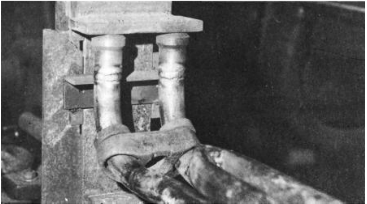
One of the elements after being welded up in the jig. The 'ball ends' which fit into the header were turned at the Society's metalwork class at Belfast Tech. (C.P. Friel)
