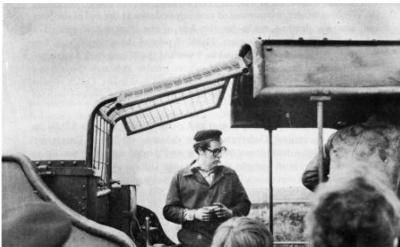
The protective 'cage' fitted to No.171 at CIÉ's request, to prevent fire irons, etc., from touching the overhead wires in Dublin. (C.P. Friel)
