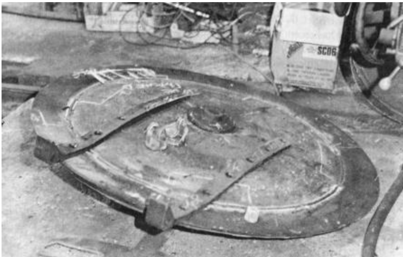
The replacement smokebox door for No.171 being manufactured. (C.P. Friel)
