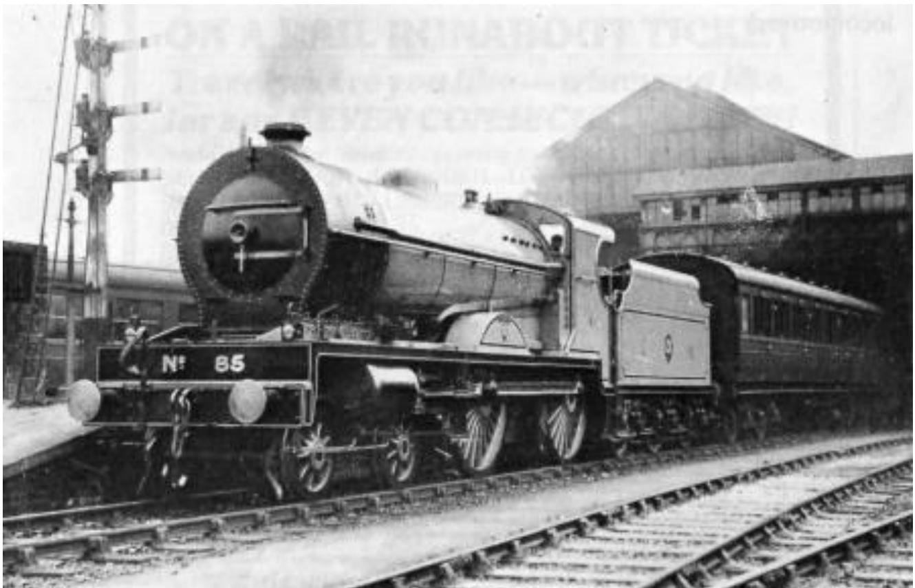
By 1938 blue livery had replaced the black. Immaculately turned out, No.85 waits to depart from Amiens Street. The sanders to the rear drivers have been removed and note how the tender side sheets have been extended to accommodate more coal. (Real Photographs X48)
