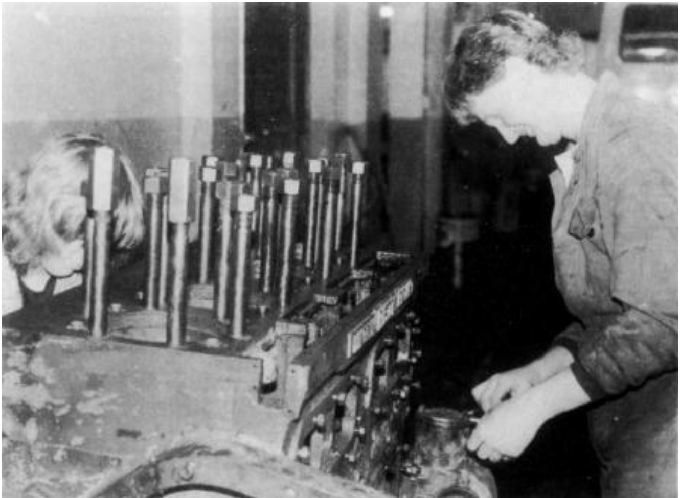
The main engine of the “Carlow Diesel” at Felden, with a forest of cylinder head studs surrounding the holes which cost £173 each to fill - see Loco Report. (I.C. Pryce)
