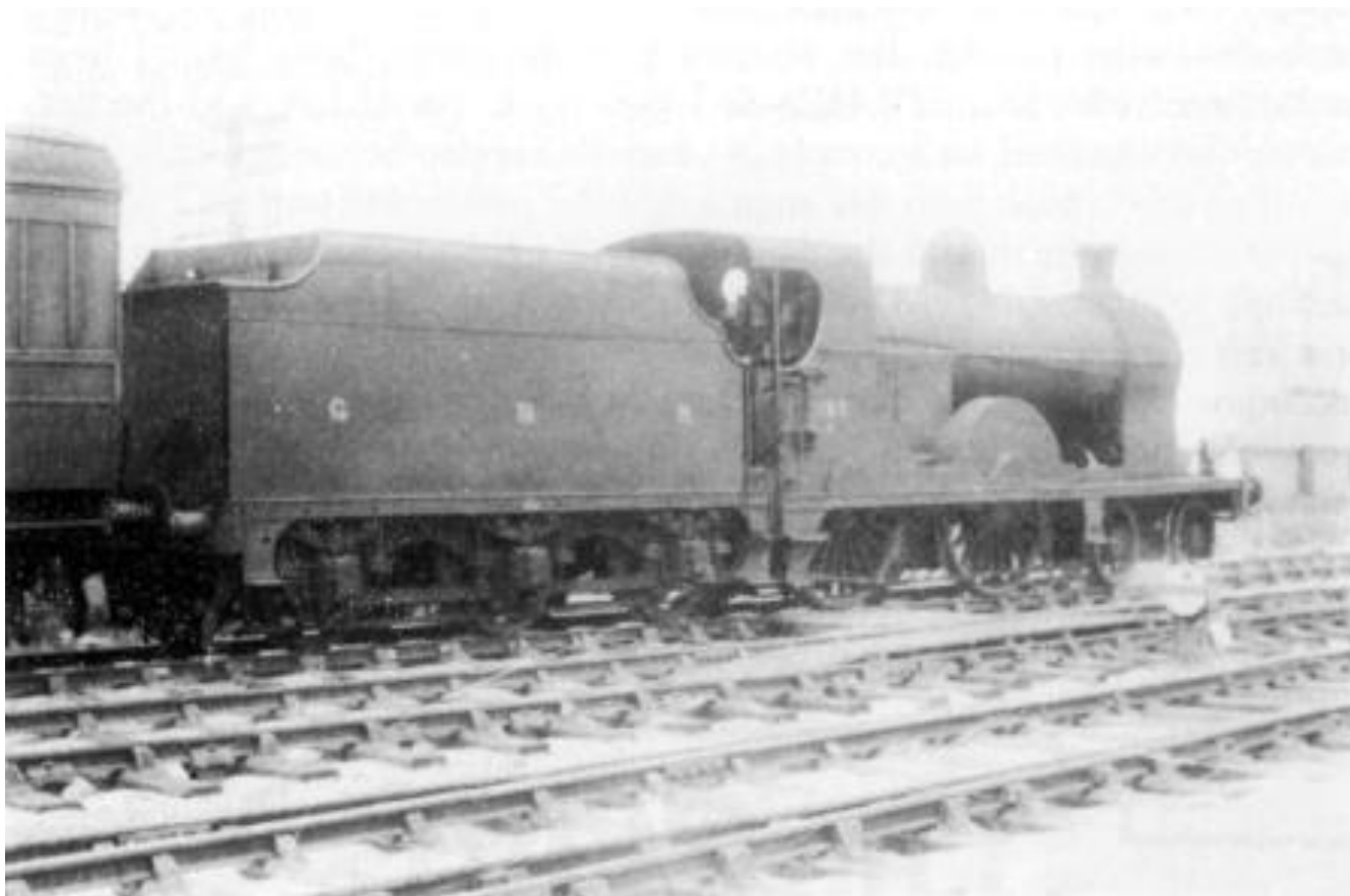
No.135 at Portrush in the summer of 1960 with a Sunday School special off the GN section. The device on the cab-side was for exchanging tablets on the NCC lines and was lowered into position by a lever in the cab. Also on the cab-side is the 'X' applied by the UTA to ex-GN locos to be withdrawn when they next fell due for overhaul and this fate befell the long-lived No.135 in the following year. (W.T. Scott)
