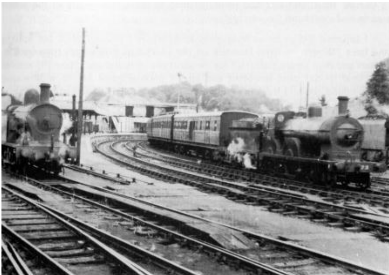
6'6" P class No.73 leaves the sharply curved station at Enniskillen in 1954. This class was similar in appearance to the PP class but, with smaller cylinders, could not match their performance. SLNCR "Lough Erne", now in RPSI ownership, is seen on the left. (A. Donaldson)
