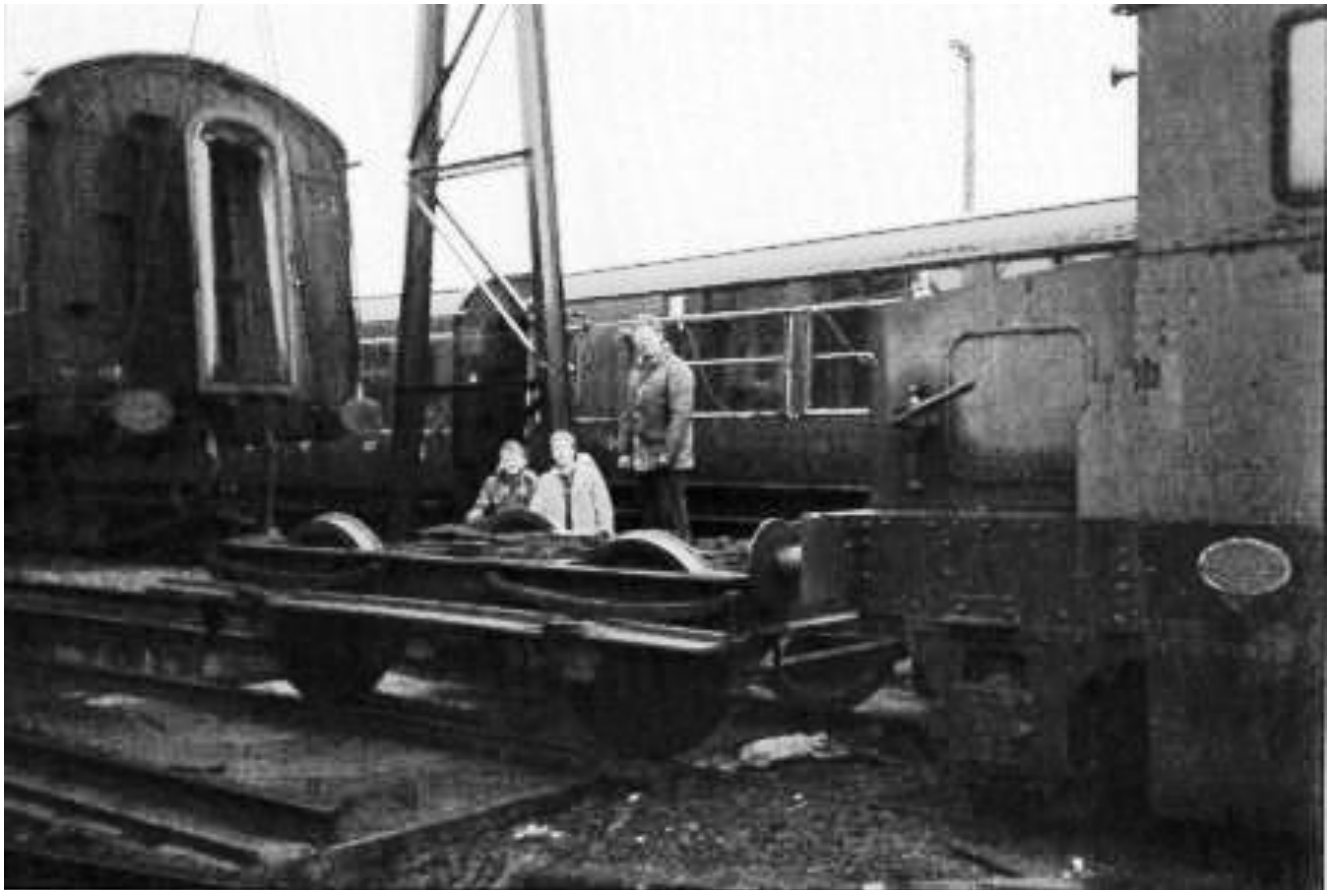
Coach 1142 under the sheer-legs for its bogie change on 21 st May 1994. (D. Mackie)
