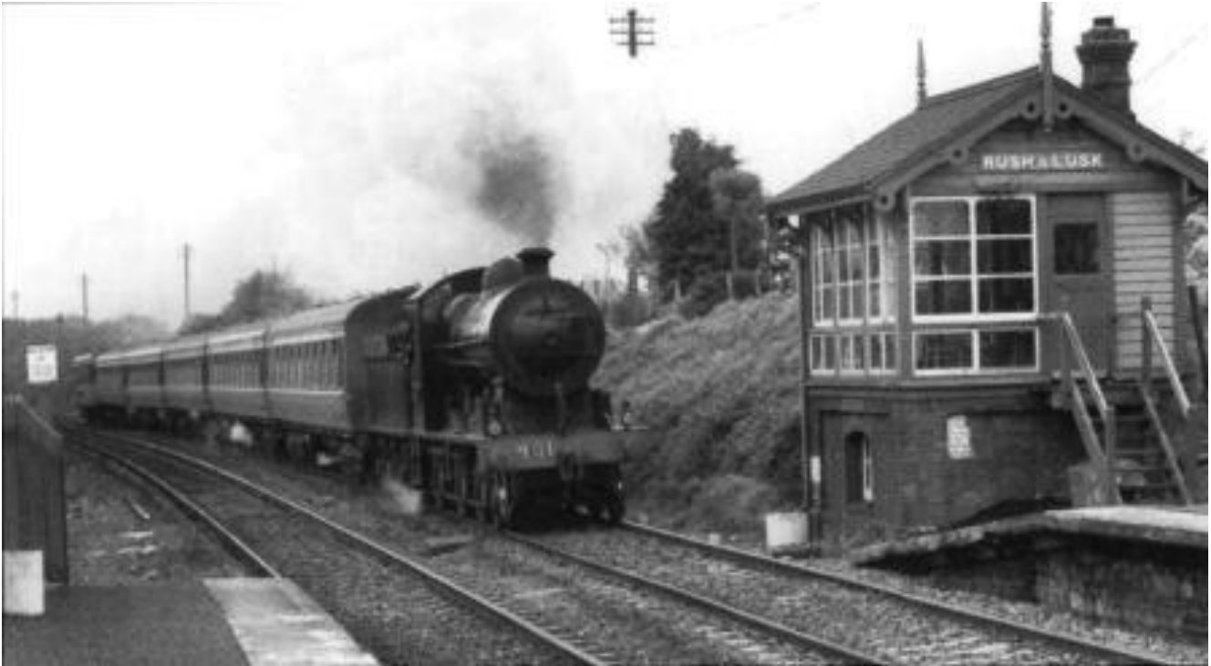
The northbound leg of the railtour on 16 th May 1994 provided opportunities to photograph some of the former GNR signal cabins, now made redundant by the extension of CTC. (C.P. Friel)
