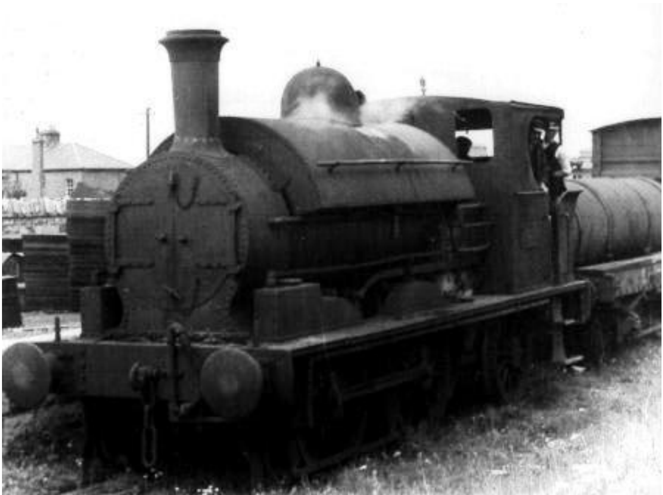
“Sambo” in 1949. The double smokebox doors were later replaced with a conventional one as the ‘duff’ era highlighted their lack of air-tightness. Note the gas cylinder wagon behind the engine. (A. Donaldson)
