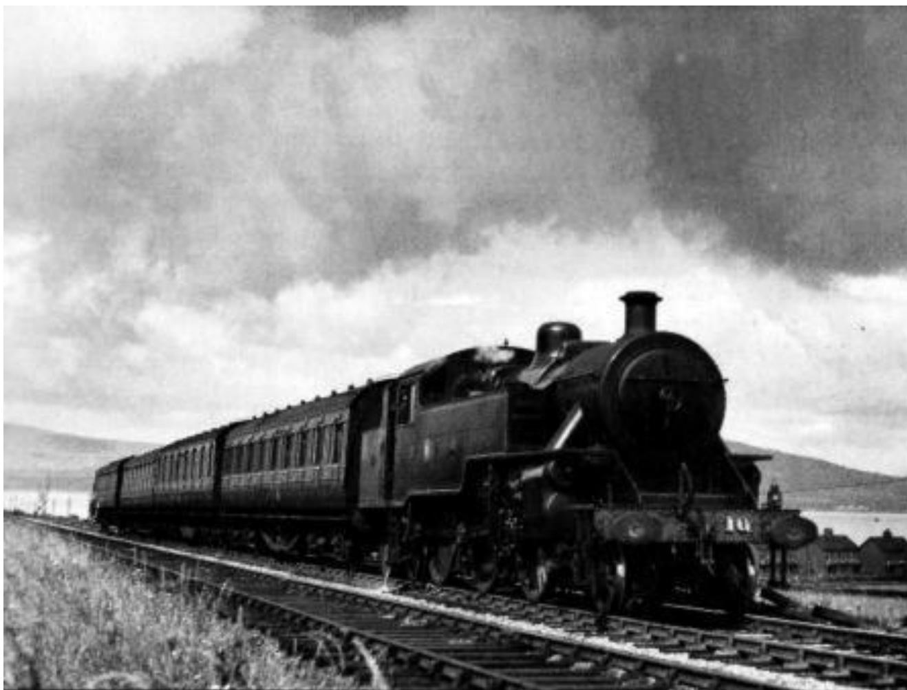
Ex-NCC 2-6-4T No.10 between Hollywood and Marino on 2 nd July 1952. With a lightweight train, the fireman is obviously taking it easy - perhaps too easy, as water is being lost from the injector. (S.C. Nash)
