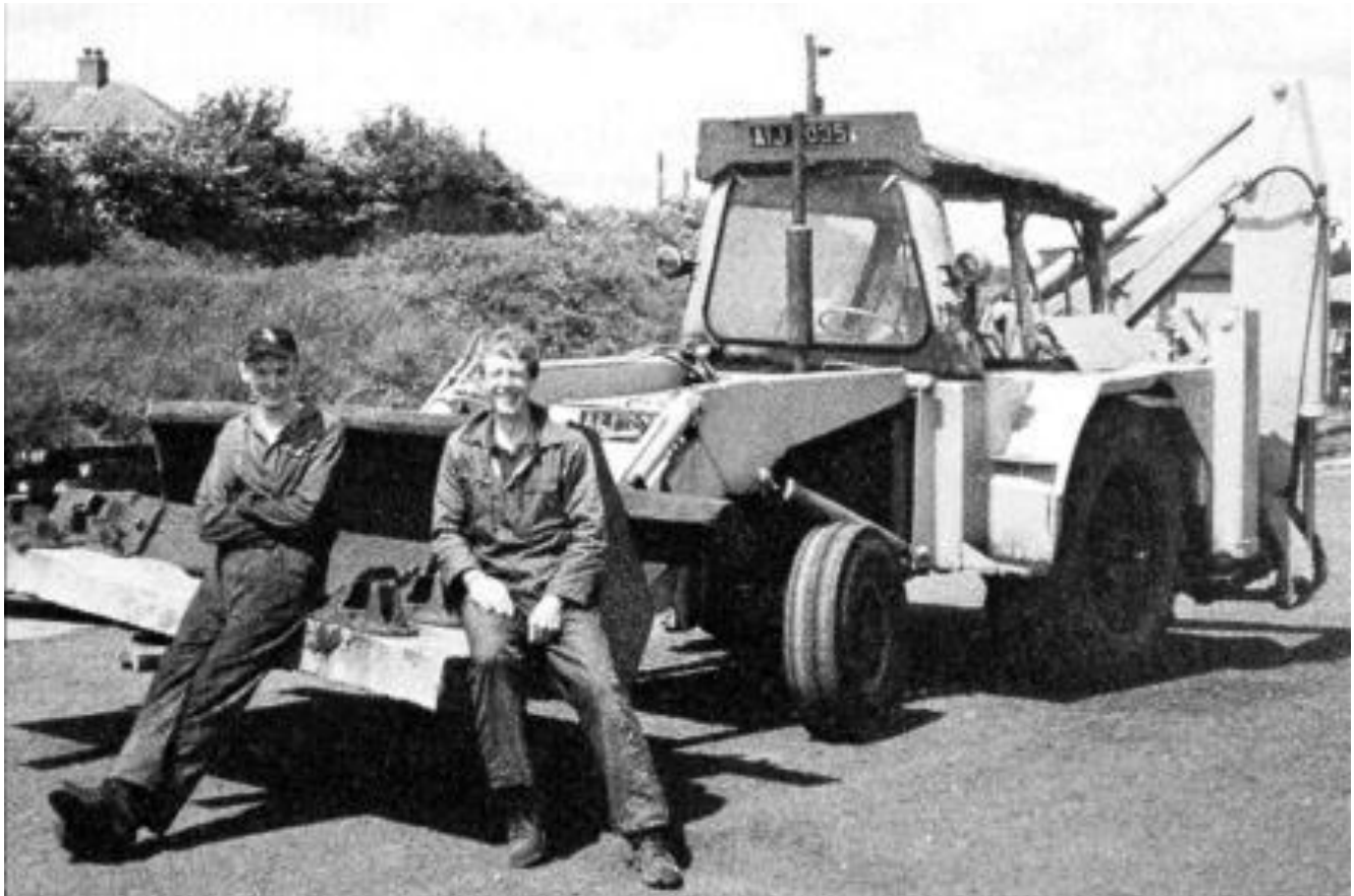
The JCB with bucket extension to carry concrete sleepers - and Philip Lockett and a Site Officer. June 1996. (D. Mackie)
