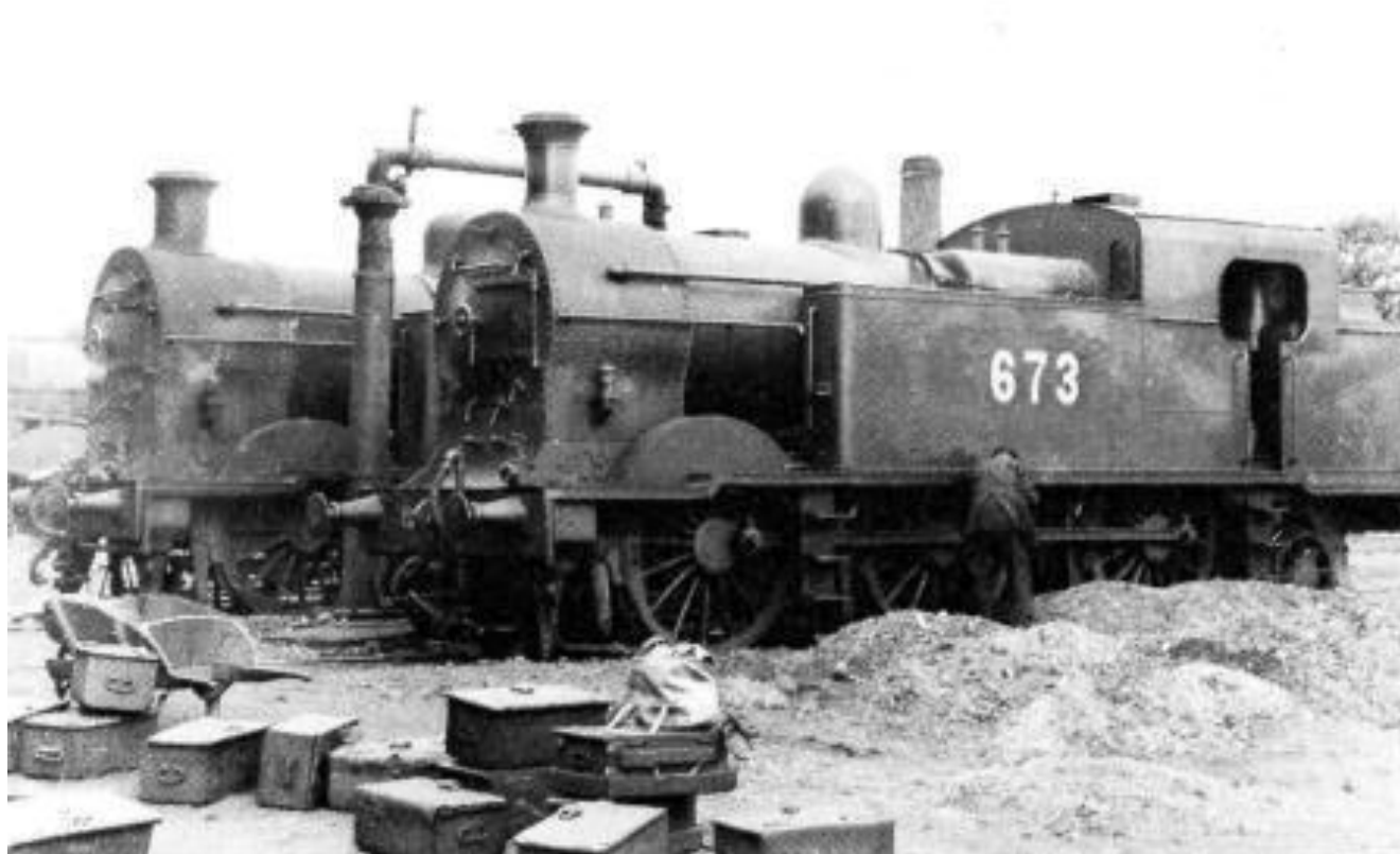
0-6-2T No.673 and No.674 (both I3 class) at Broadstone in 1959. They are said to have been somewhat lifeless compared with the GNR or BCDR suburban tanks. The containers in the foreground appear to be locomotive tool-boxes or lockers but why are they strewn around the yard? (W.T. Scott)
