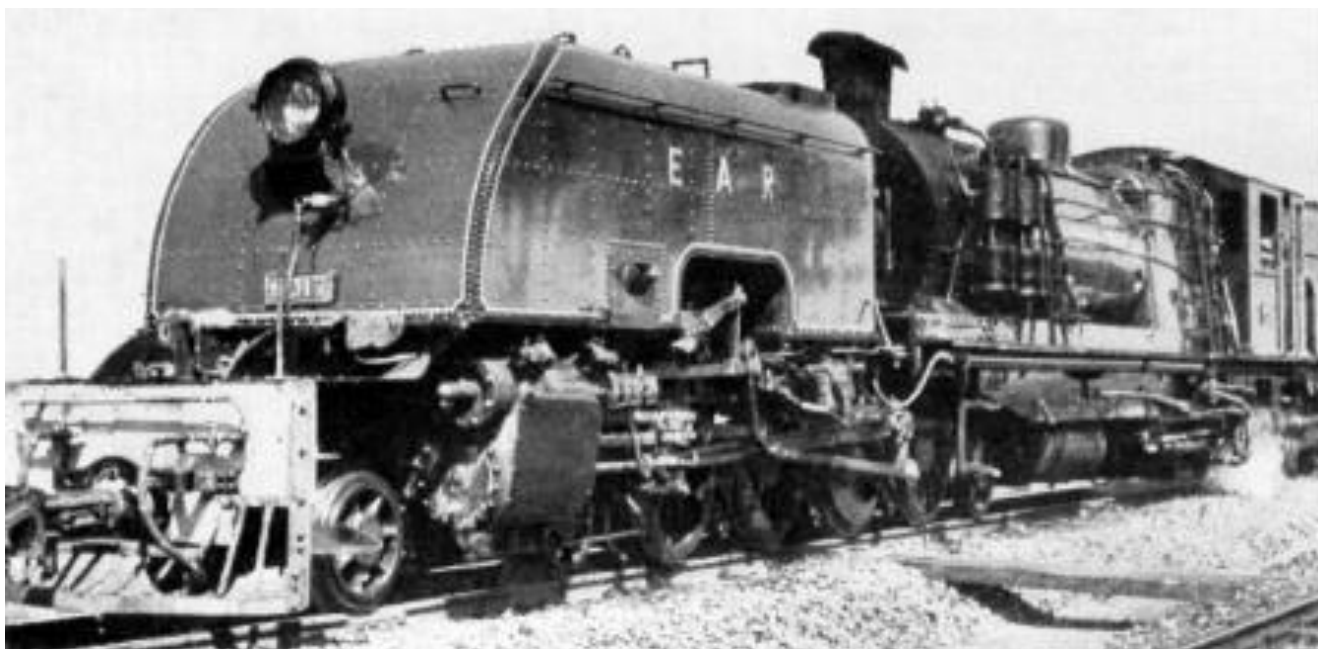
6017 "Sir John Hall", showing the less angular tank also carried by the 56 and 59 classes. Also plain to be seen is the rather unsightly chimney which accompanied the Giesl ejector fitted to almost all EAR locos from 1961 onward. (D. Ramaer collection)
