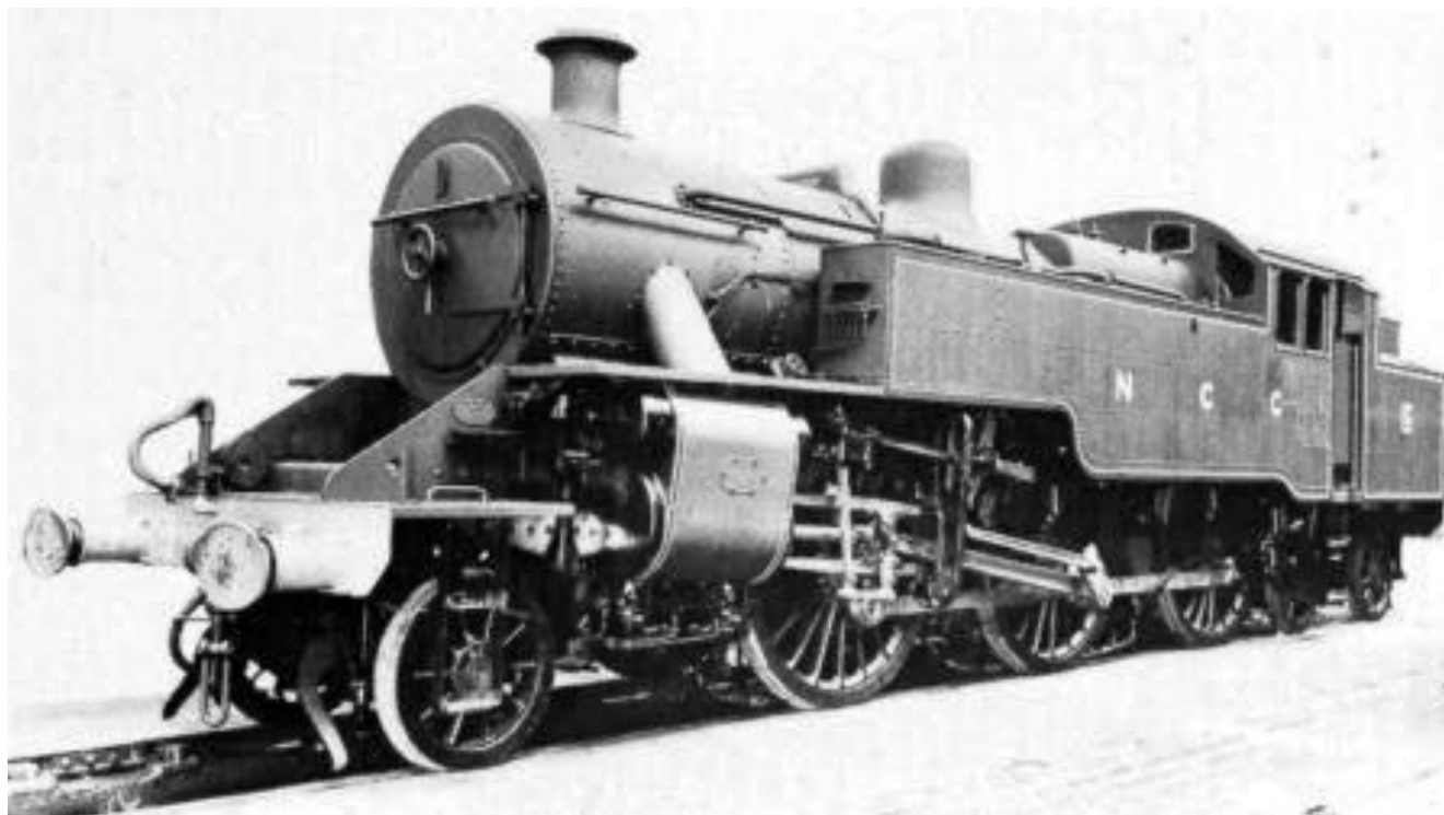
2-6-4T No.5 in new condition in NCC livery. The lever for the hopper ashpan can be seen midway along the rear coupling rod. (Real Photographs Ltd)
