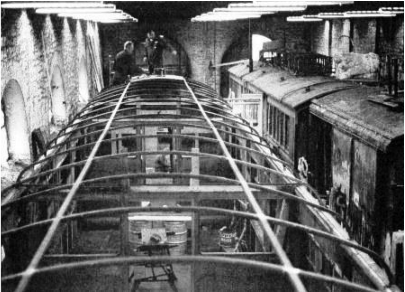
Paddy O'Brien and Denis McCabe at work on 1463, the last surviving laminate coach in the Dublin fleet, under overhaul at Mullingar. Note the new steel roof members. (P. O'Brien)
