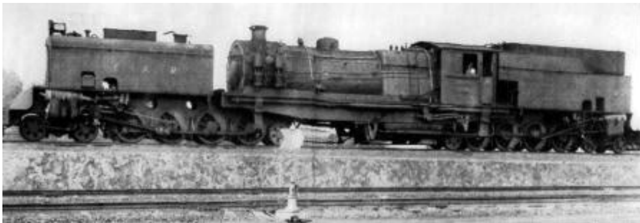
5302, the Garratt which almost managed to travel on two lines at once. The photo clearly shows the boiler and cab pivoted between the two power units. The twin Westinghouse air pumps are mounted beside the smokebox - how would one of these look on 171?! (D. Durrant)
