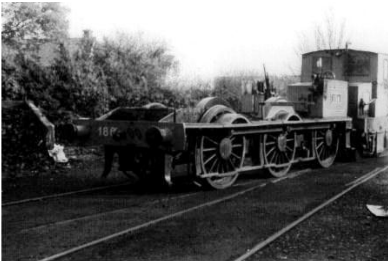
No.186 did not rest long at Whitehead before its boiler was removed for inspection. Here the long-suffering diesel No.23 propels the remainder into the loco shed. (P.A. Scott)
