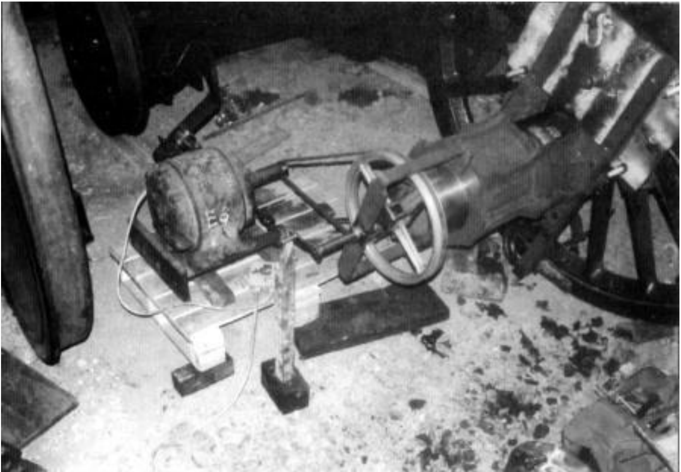
Whitehead's latest in-house product - the crankpin machine - in action on one of No.4's driving wheels. The driving belt tensioner is not fully visible but consisted of a chain hoist attached to the guard iron of the pony truck in the background! (P.A. Scott)
