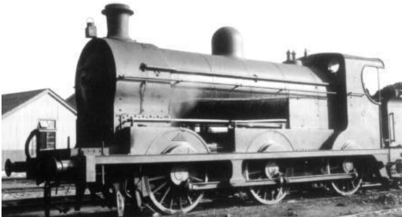
SG2 No.19 at Dundalk shed in 1936; note Nasmyth Wilson builder’s plate on the leading splasher. A pity to spoil its delightfully clean lines by not using a few more inches of piping, thereby allowing the oil pipes to run parallel to the handrail! (Loco & General)
