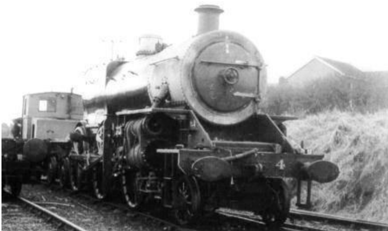
Partly assembled No.4 is transferred from the shed to the loco workshop for trial fitting of tanks, bunker and cab. (I.C. Pryce)
