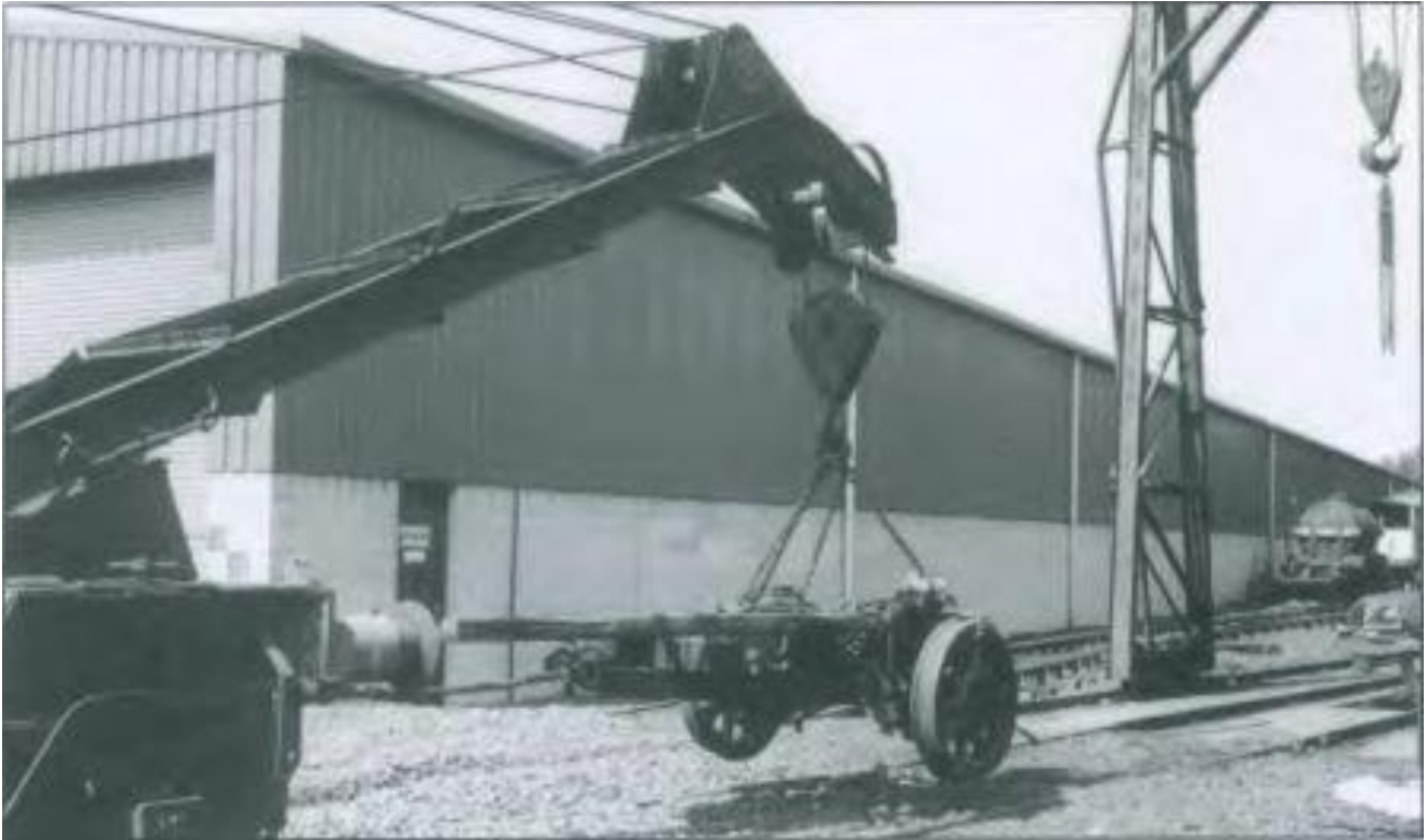
Not a field gun, but No.4's pony truck with a large piece of wood on top, being positioned for the re-wheeling of the frames. (P.A. Scott)
