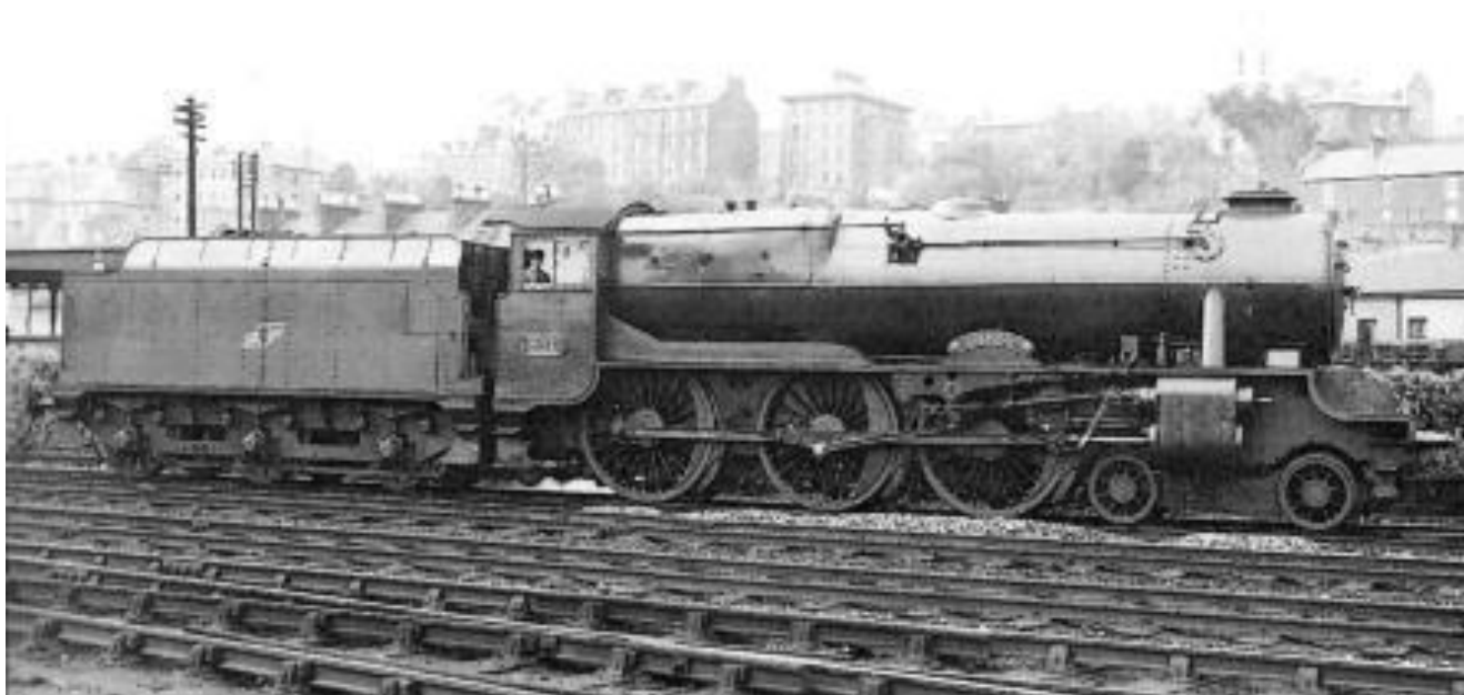
No.800 at Cork in 1949. Although the boiler was parallel, its cladding was tapered. The graceful lines were somewhat marred by the outside rodding to the regulator from the duplicating levers in the cab. One might have expected the rodding to have been on the driver's side, resulting in less potential slack in the linkage. (Sean Kennedy)
