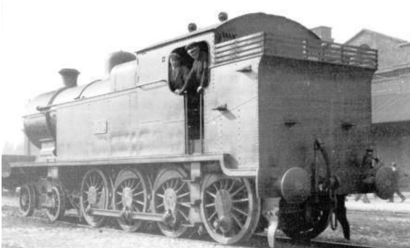
GSW 4-8-0T No.900, showing its conversion to a “Pacific” wheel arrangement. By coincidence the crank pin of the rear wheel is “in step” with the others. (I.C. Pryce collection)
