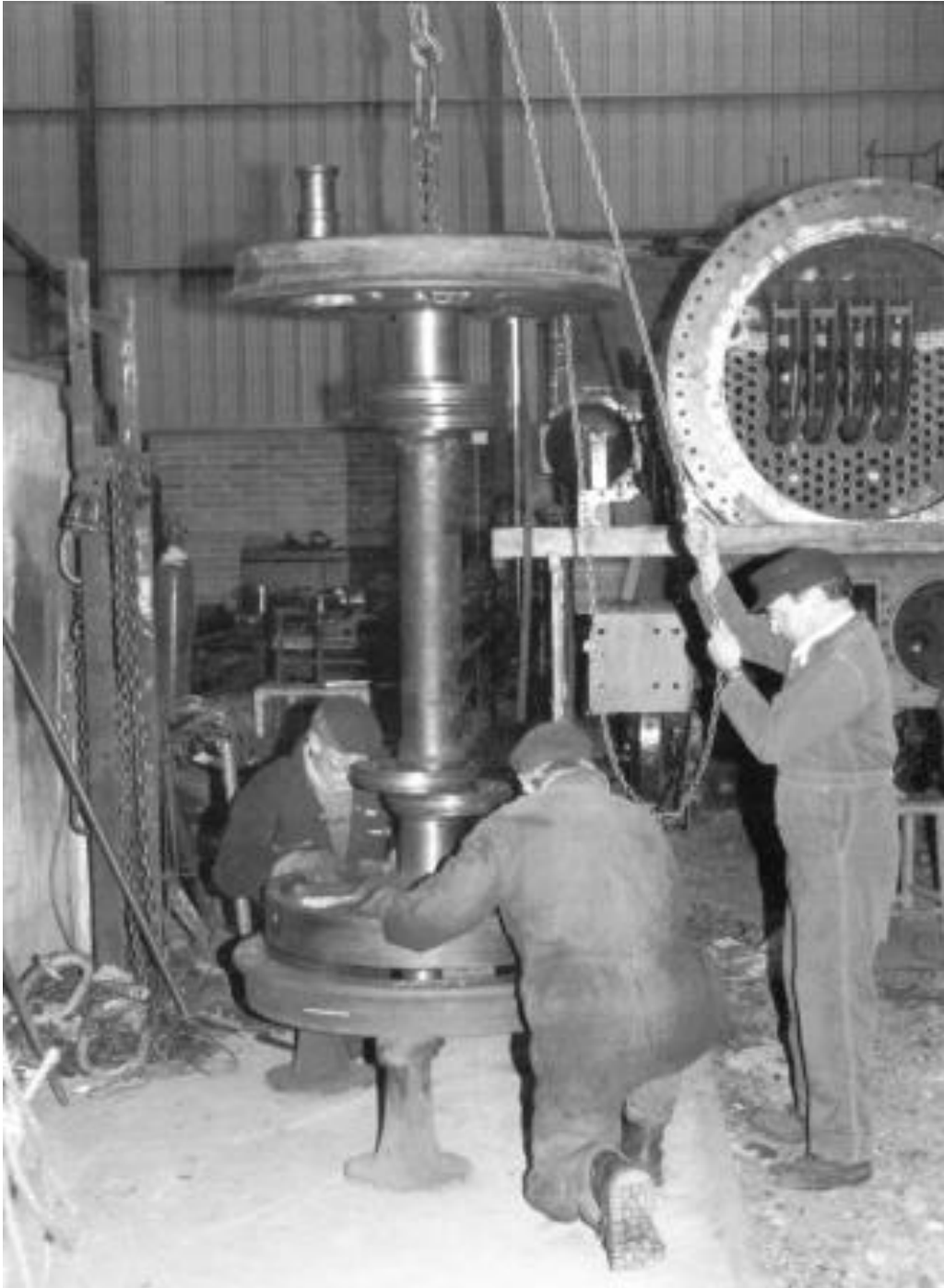
Repairs having been completed, BG3's tyre has been expanded by heating and the wheelset is being lowered into it. On the right, the new boiler tubes and superheater elements fitted to No.186 can be seen (I.C. Pryce)
