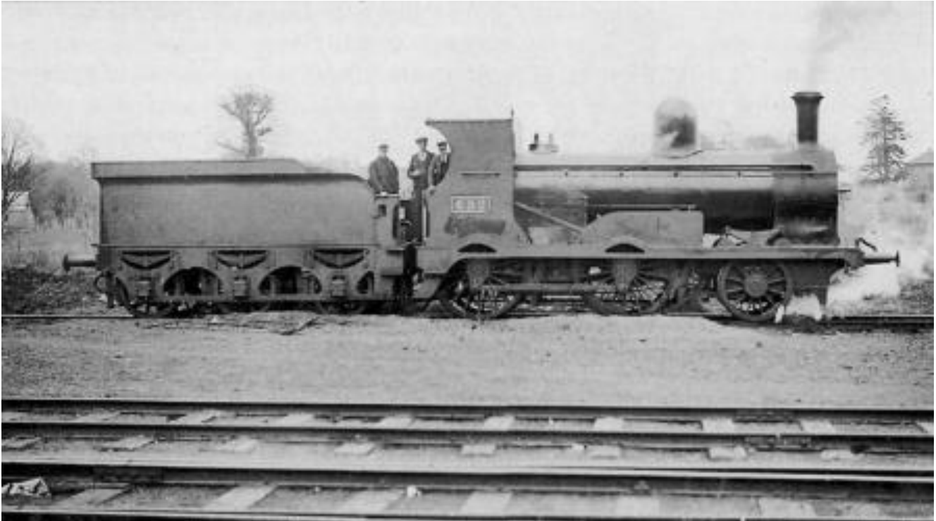
No.652 at Kingscourt in 1938. These were by a long way the last 2-4-0 locomotives to work in the British Isles. (A.W. Croughton/W.T. Scott collection)
