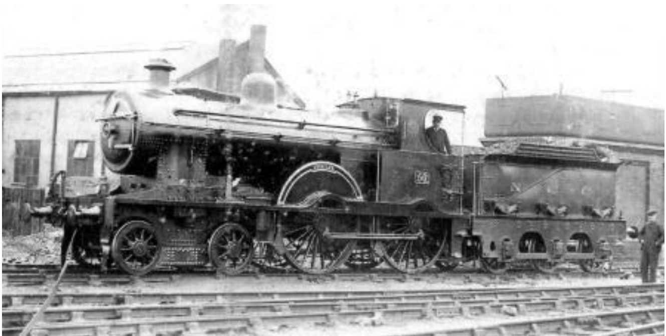
After being twice rebuilt (the BNCR/NCC were notorious rebuilders and renumberers), No.50, still "Jubilee", is seen here in its final 4-4-0 form at Belfast York Road c1930. The locomotive was finally scrapped in 1946. (W.T. Scott collection)
