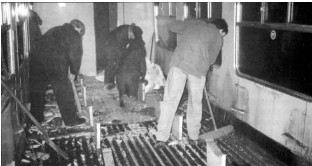
A very open Mk2, with all interior furnishings stripped out prior to re-panelling and painting. The floor covering will also be replaced, and here the old material is being removed. (J. Wolsley)
