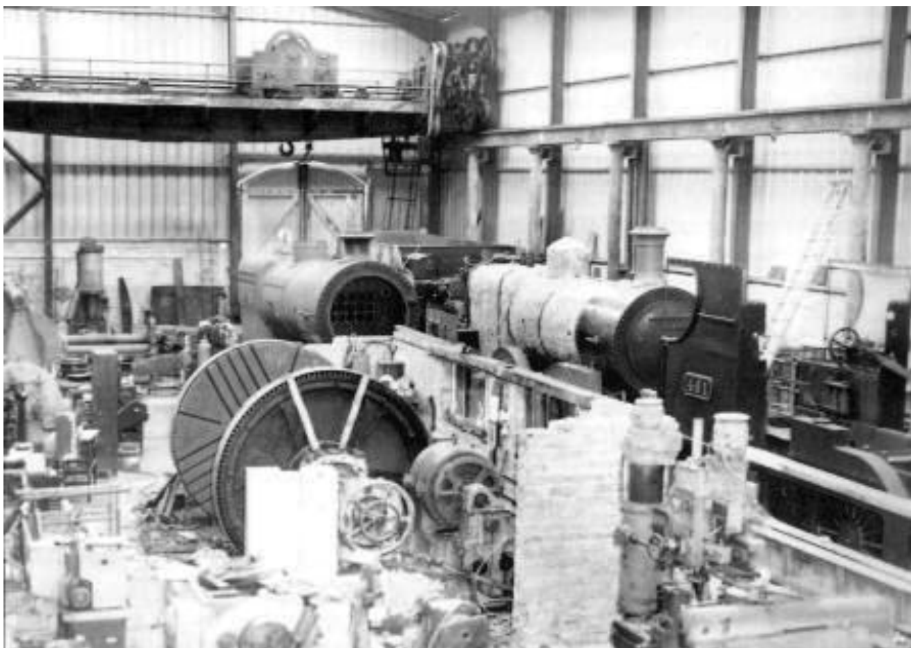
Locomotive Workshop, October 2003, left to right: No.461's boiler, No.186 awaiting cab and boiler cladding, remainder of No.461. To the right of the wheel lathe in the foreground are the remains of the house it used to occupy before the workshop was built. (C.P. Friel)
