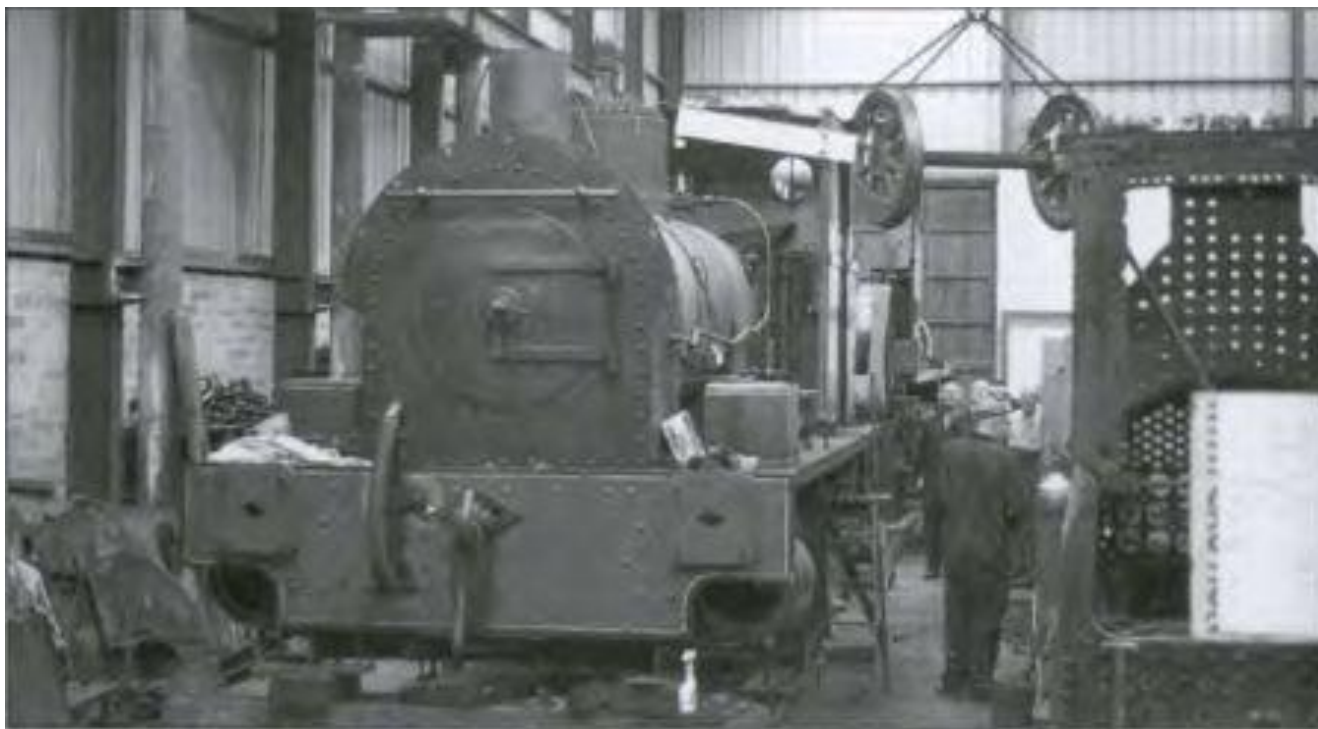
The “Derry Engine” in the latter stages of its overhaul in the workshop at Whitehead, its wheels being craned onto the rails. A temporary chimney has been fitted for steam testing and the white board clamped to the cab carries a pressure gauge on its other side! On the right is the inverted firebox of No.461, on which the missing platework has since been replaced; the board here had a “things to do” list for No.3. (I. Pryce)
