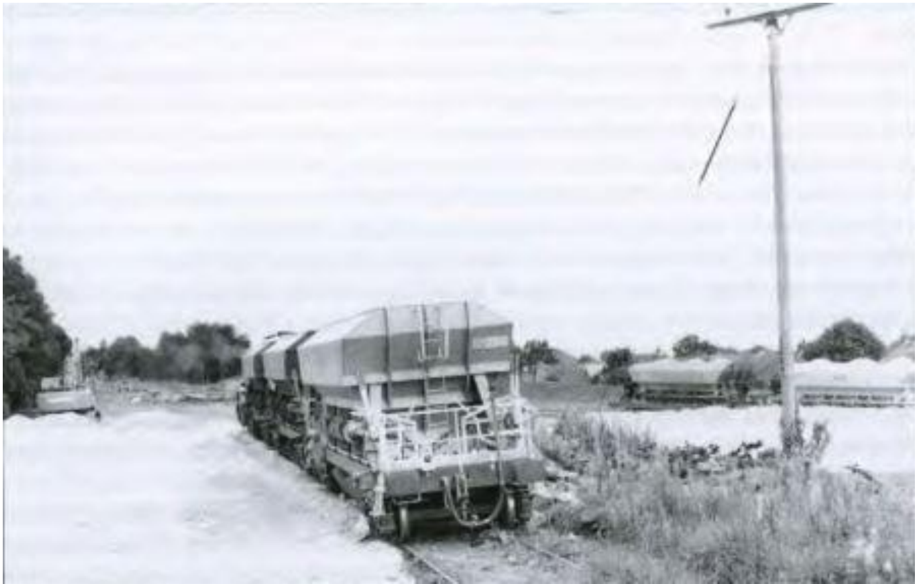
A quiet day at Greenisland - loaded wagons on the Down line and No.3 awaiting instructions on the Back line with not a soul in sight except the fireman. The tail pipe and vacuum brake application valve can be seen on the rear of the nearest wagon. (C.P. Friel)
