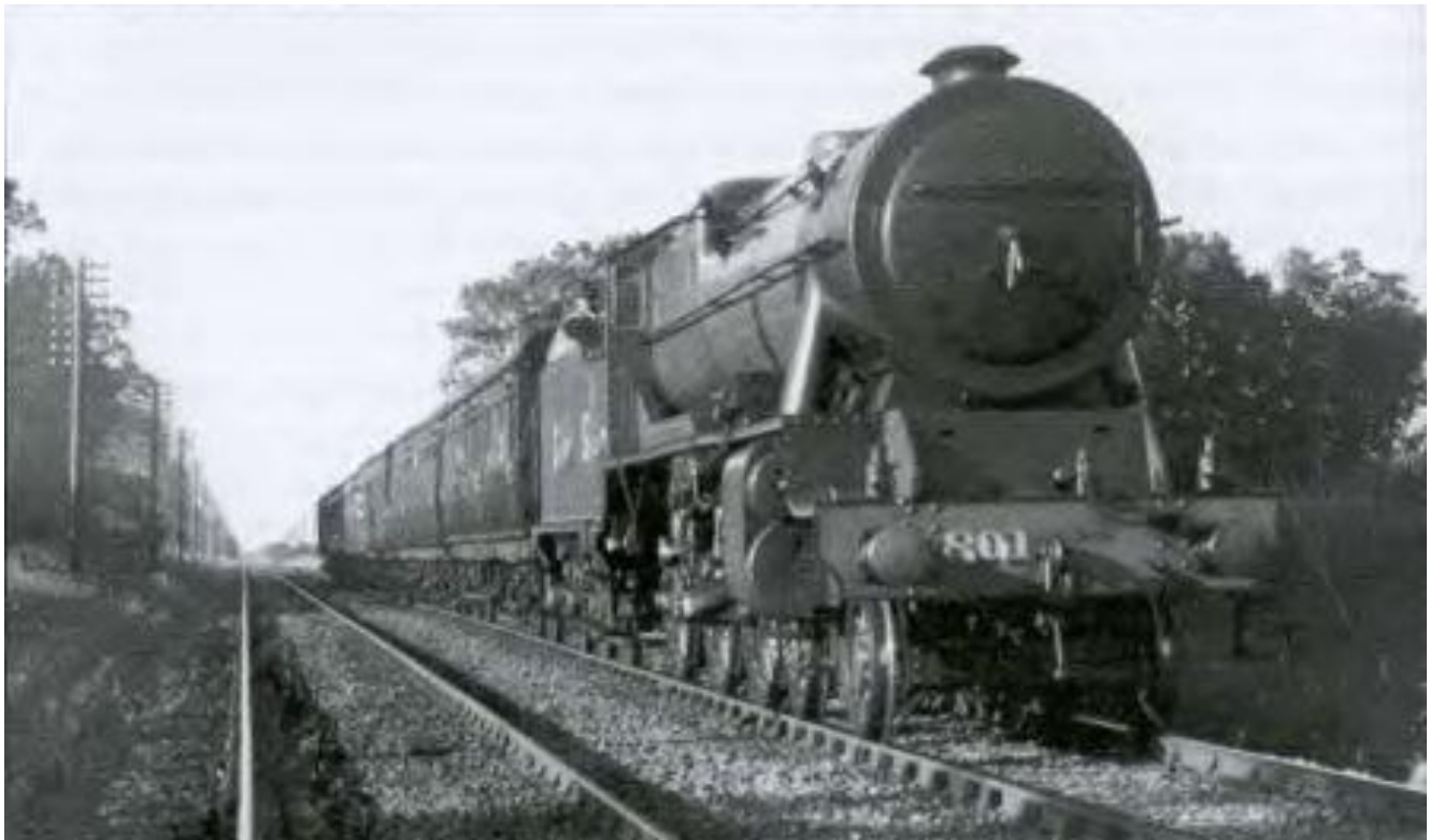
No.801, as yet un-named, with a test train near Templemore in 1940. A bowler-hatted inspector is in the fireman's seat and below him the drive for a speedometer can be seen mounted under the running plate. Can anyone comment on the coach behind the engine? (S. Kennedy)
