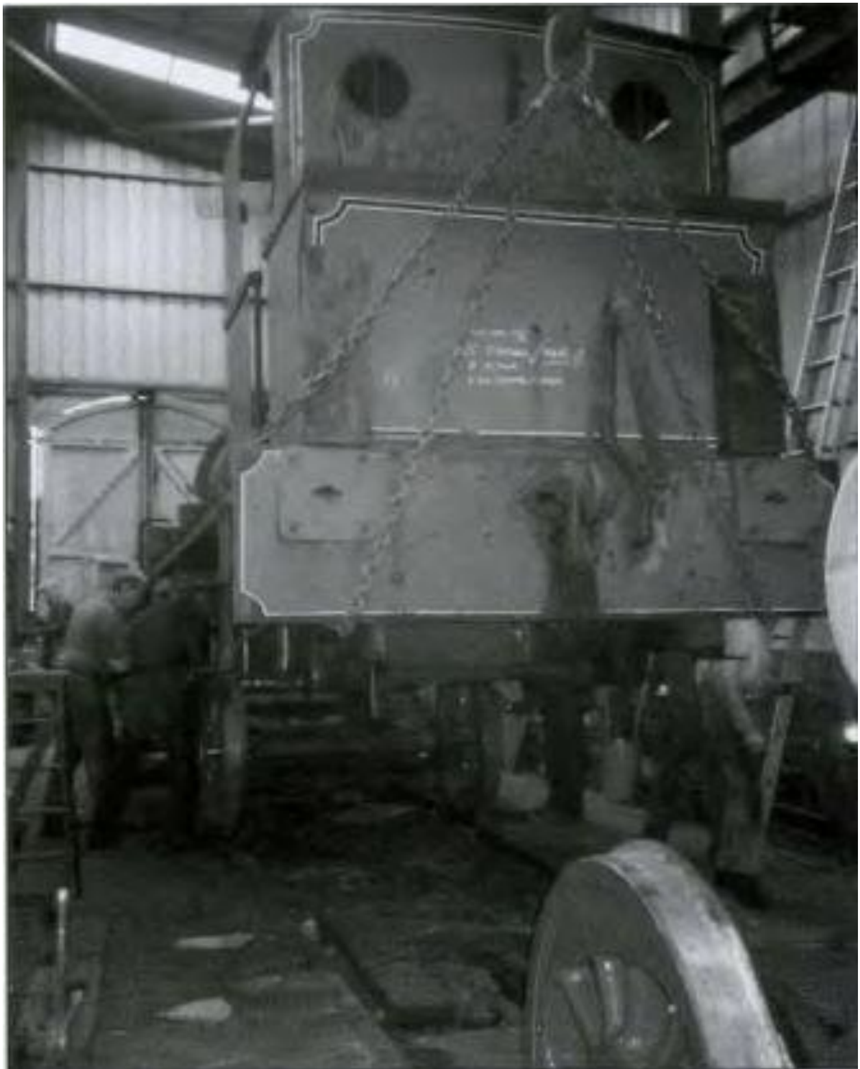
With its front end supported on blocks, No.3 is now raised to enable the wheelsets to be rolled into position. (J. Wolsley)
