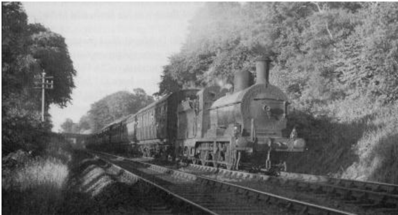
PG No.103 with an excursion train near Craigavad c.1959. Although built as goods engines their light axle load enabled them to work to Bangor via the “Shaky Bridge “ over the River Lagan. (W.T. Scott)
