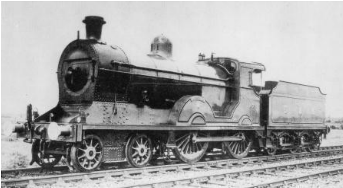
S class No.190 "Lugnaquilla", newly painted in blue. Note inside-keyed track in foreground. (Real Photographs/C.P. Friel collection)
