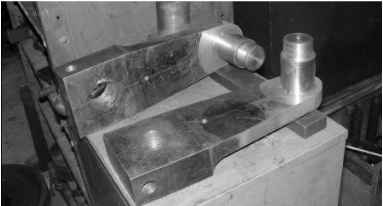
How many preserved railways do this? Return cranks for “Drumboe” forged and machined at Whitehead. (J.J. Friel)
