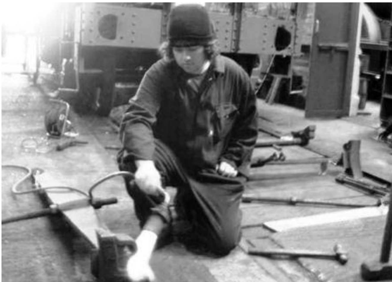
Ben has landed a nice warm job, freeing up parts of the brake gear. (J.J. Friel)
