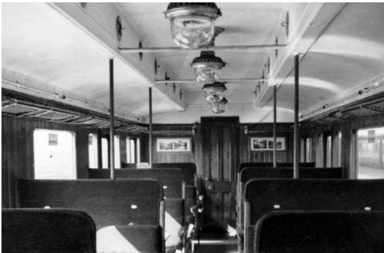
More luxurious than the coach described by the author but showing the glass bulbs of its gas lamps, this is CIÉ clerestory 819, a 50ft saloon third built in 1901 and withdrawn in 1960. (M.H.C. Baker)
