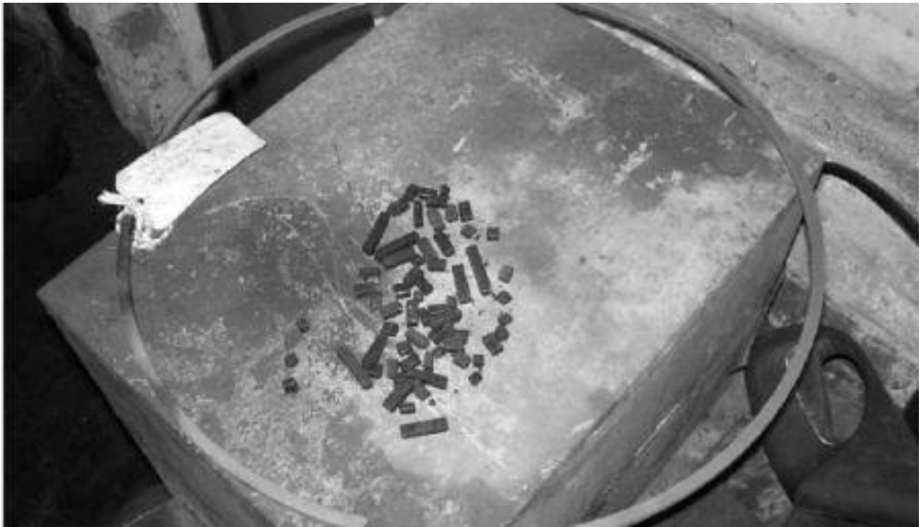
One of No.4's piston rings - and the remains of another! (P. Scott)
