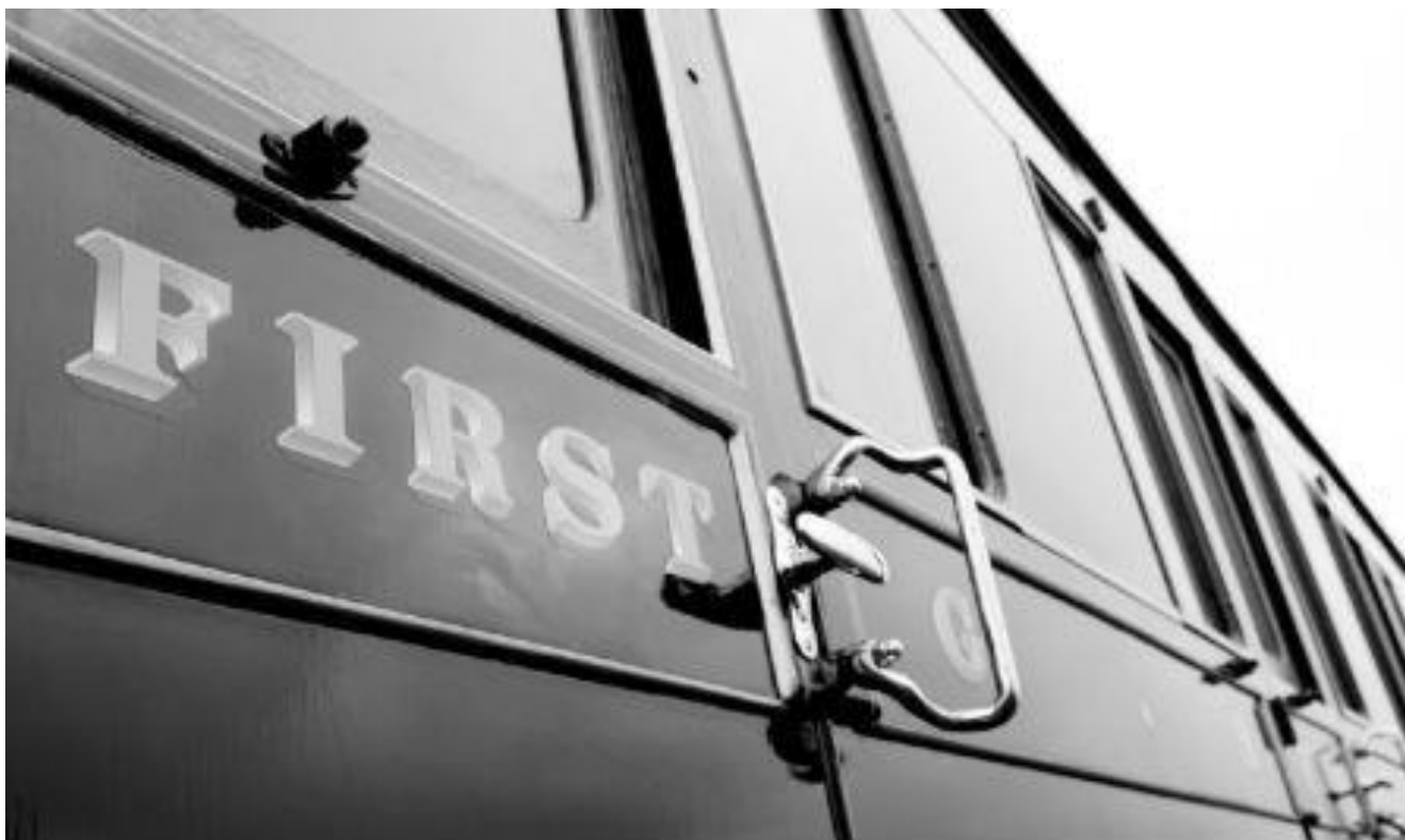
Detail of lettering, also note the substantial and re-chromed door and grab handles. (C. Meredith)
