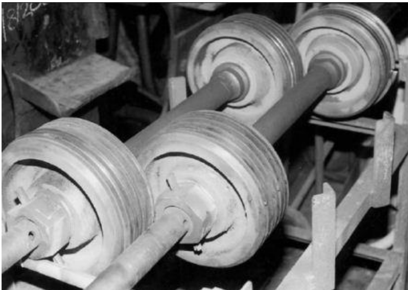
No.4's valves after refurbishment, showing the multiple rings which tend to become jammed by carbon deposits. (I.C. Pryce)
