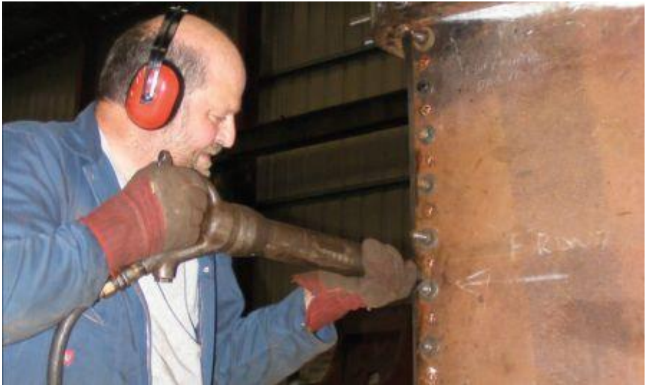
With No.461's inner firebox inverted and plates held by temporary bolts, Bob Skingle tackles the hot and noisy job of riveting. (C.P. Friel)
