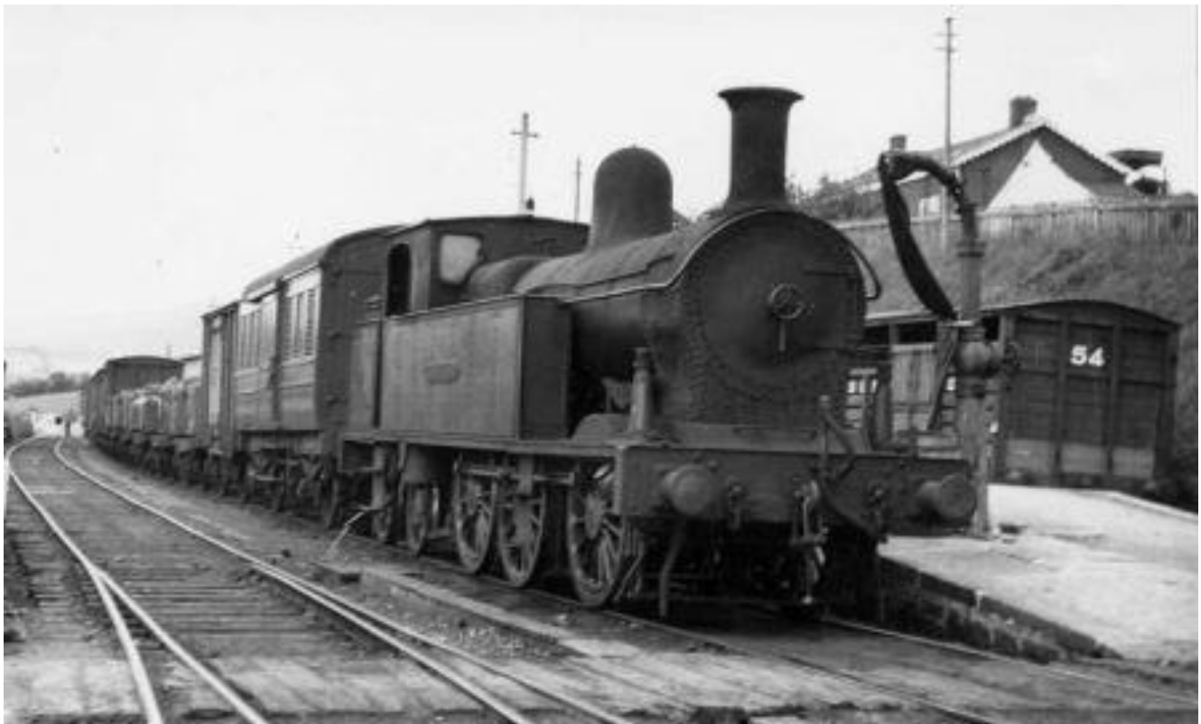
SLNCR 0-6-4T “Enniskillen” at Manorhamilton on 10 th June 1950 with the 14:00 down goods. Mr Egan’s house can be seen on the right. The SLNCR appeared wedded to this design which originated in 1882 and continued, with only slight alterations, up to “Lough Erne” of 1949, now part of the RPSI collection. (W.T. Scott)
