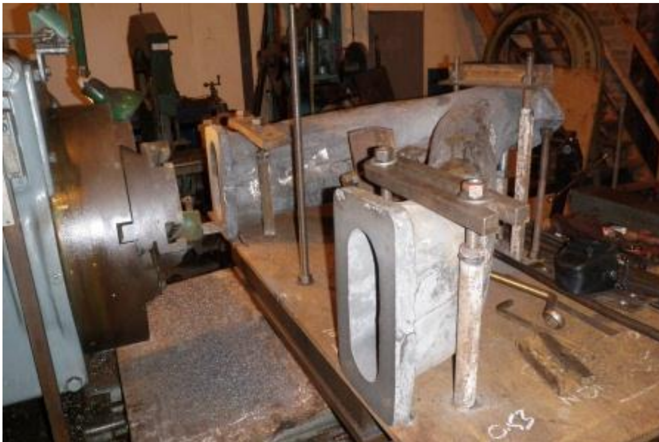
The flanges of No.85's newly cast blast pipe being machined. The hardest part of this operation was getting the work accurately set up. (P. Scott)
