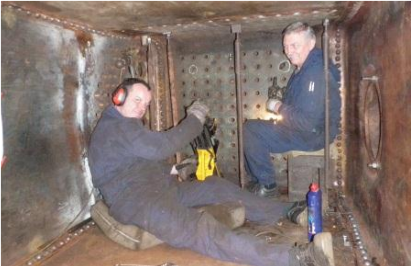
With No.461's boiler lying on its right hand side, Jim Adams and Billy Clements work on crown stays. At that stage, 9 th June 2010, there were still many more stay holes to be drilled and filled. (P. Scott)
