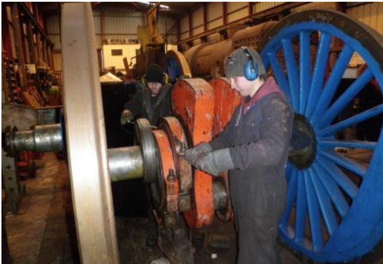
Whitehead apprentices James Spurler and Michael McCann at work on No.85's eccentrics. As that is not a noisy job their headgear would suggest that riveting is taking place nearby. (P. Scott)
