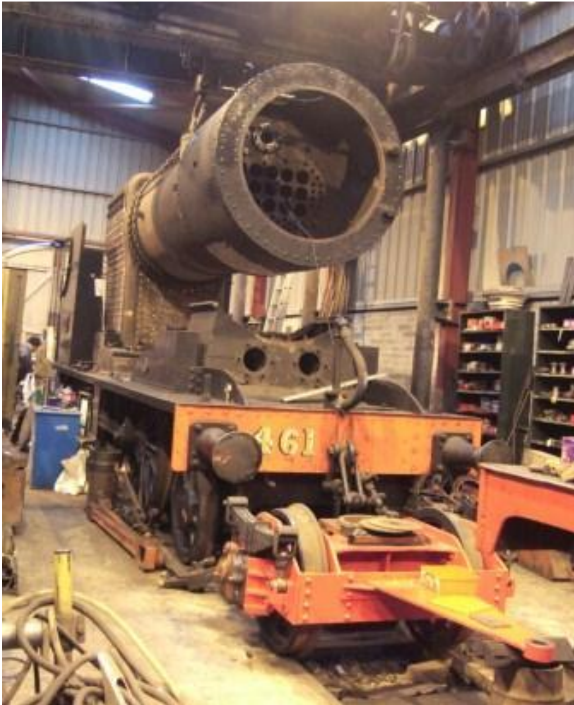
No.461's boiler is lowered into the frames for trial fitting on 15 th January 2011. (P. Scott)
