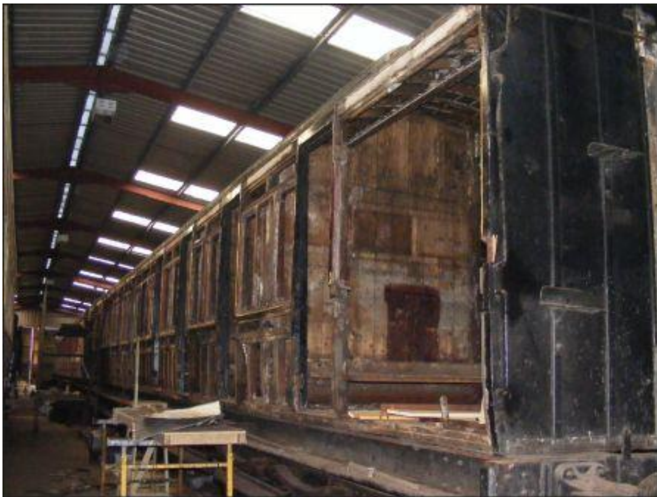
The quest to find good wood in GS&WR carriage 861 has involved losing a lot of material, as seen here on 19 th April 2011. (E. Friel)
