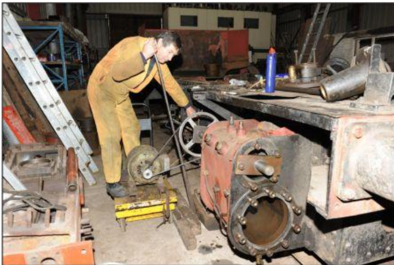
Jeff Spencer boring out the valve liners of O&K No.1 on 20 th July. (R. Edwards)
