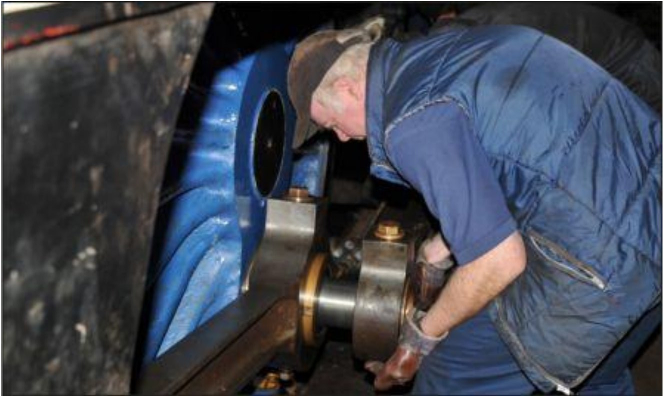
Thomas Charters (with helpers!) re-fitting No.85's refurbished left connecting rod on 5 th November 2011. (C.P. Friel)
