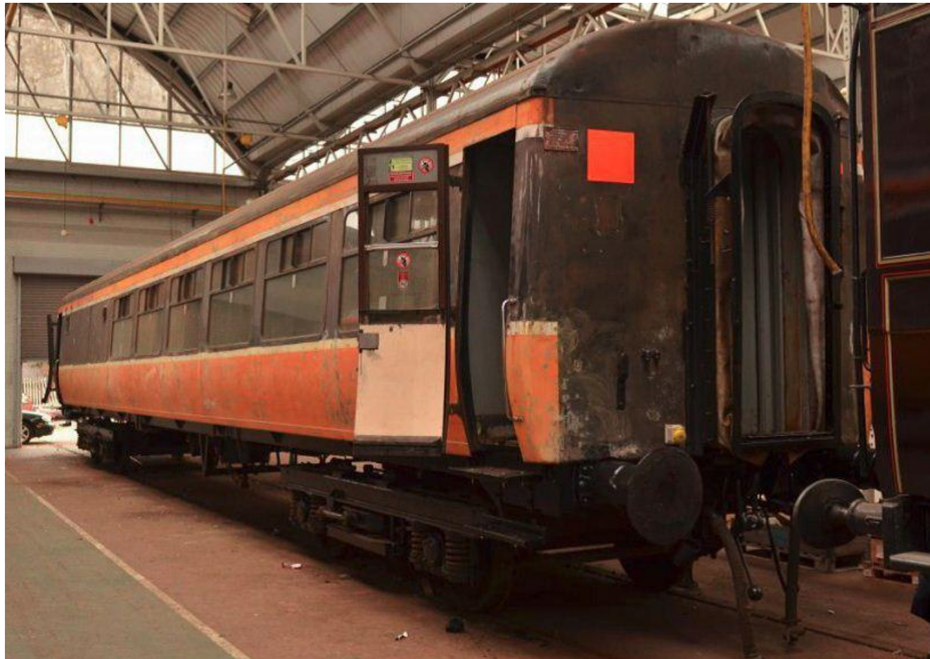
Former buffet car 1508 in the midst of its overhaul in the former Carriage One shop at Inchicore, February 2013. When converted to a catering vehicle, two windows were plated over on one side, giving it a rather distinctive appearance. (L. Tomiczek)
