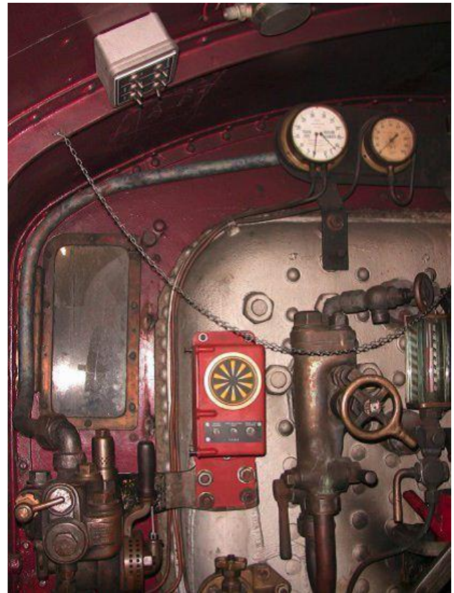
An all-new electrical system is being installed (left) including TPWS, which gives warnings to the driver through a horn, a bell, and a 'sunflower' indicator (centre of right-hand picture).
