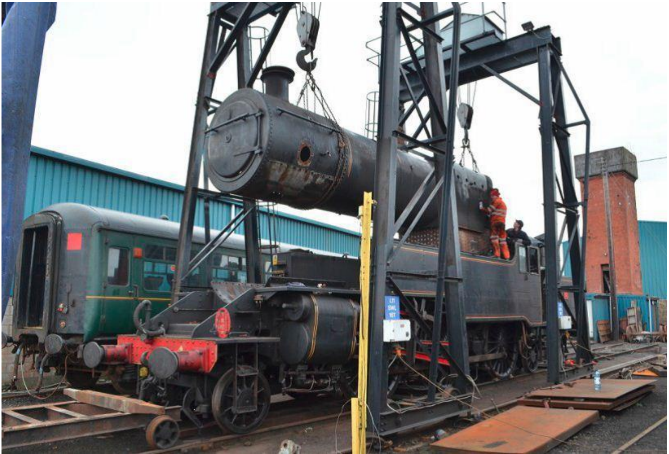
No.4's boiler is removed for inspection on 14 th March 2013. (A. Lohoff)
