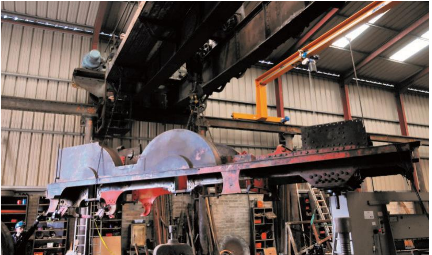
On 26 th April 2014, No.131's frames were rotated through 180 degrees to face the same way as the boiler. The locomotive is being assembled with the chimney facing Larne.
