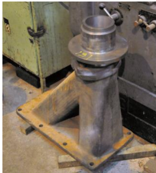
The new blastpipe, which was cast at Whitehead.
