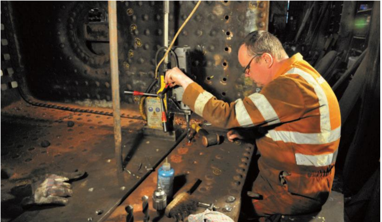
Jim Adams of HEI drilling stay holes in 131's firebox in May 2014.
