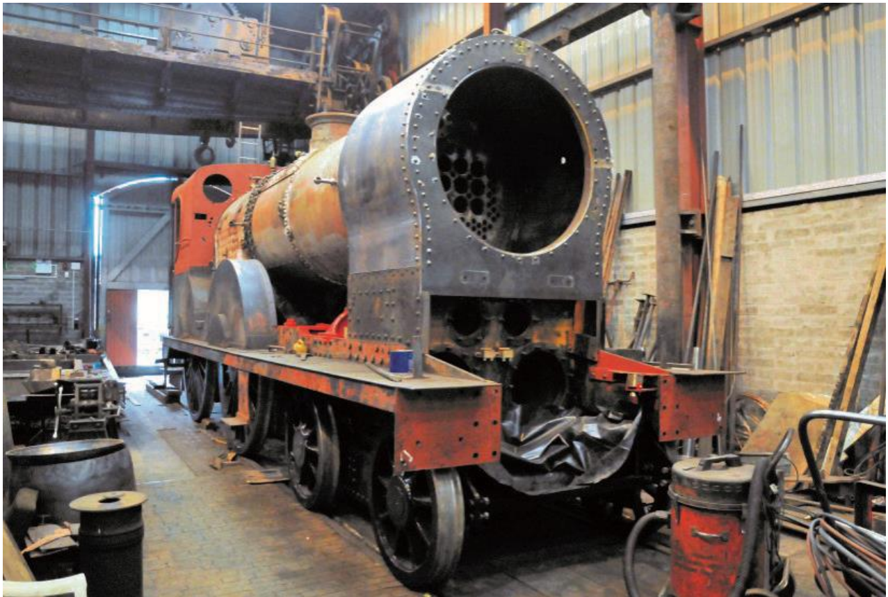
In September 2014, No.131 is seen having the boiler, along with the new smokebox, temporarily test fitted. It is vitally important that this project is completed on time so all volunteers are welcomed!
