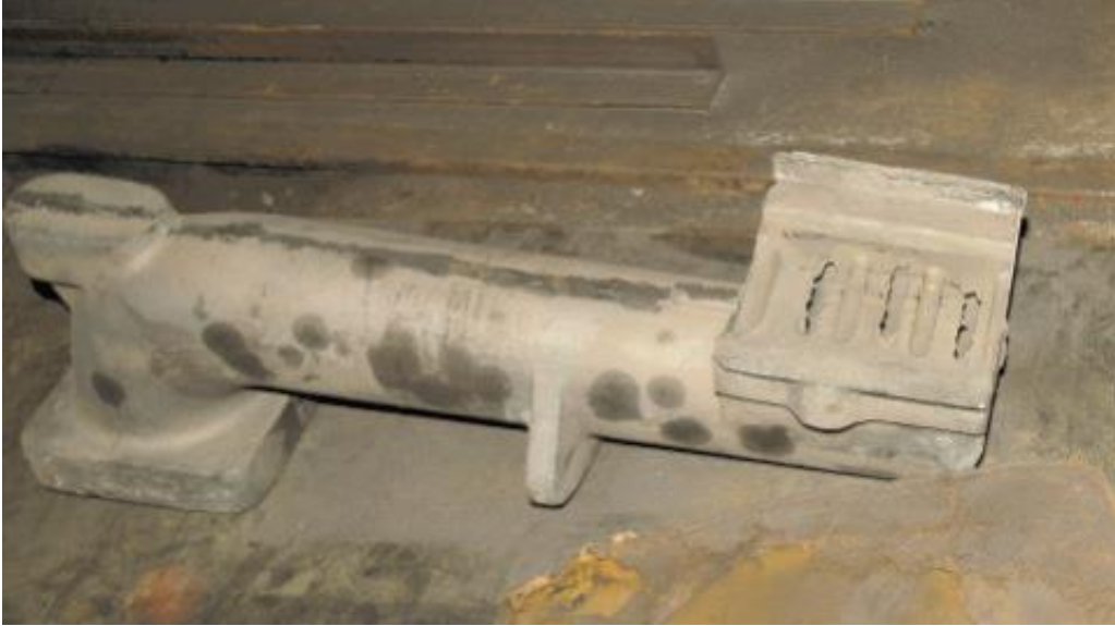
This component, newly cast in the Whitehead foundry, forms one half of the regulator
