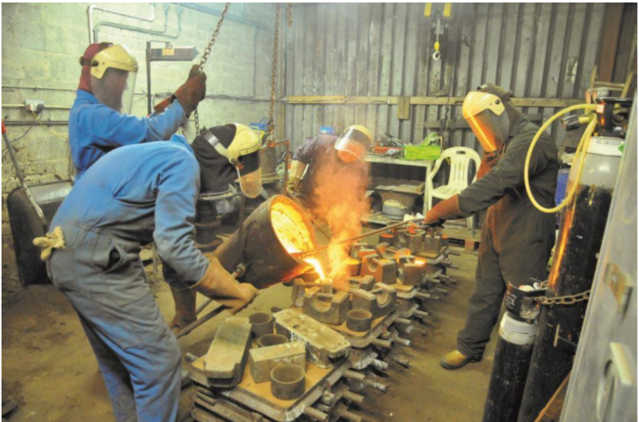
Casting brake blocks in the old Whitehead foundry, January 2015. Top left: making moulds; above: pouring molten iron; top right, the resulting rough casting. The foundry - a lean-to building behind the engine shed - has now been demolished to make way for a much larger workshop building, which will incorporate a new foundry.
