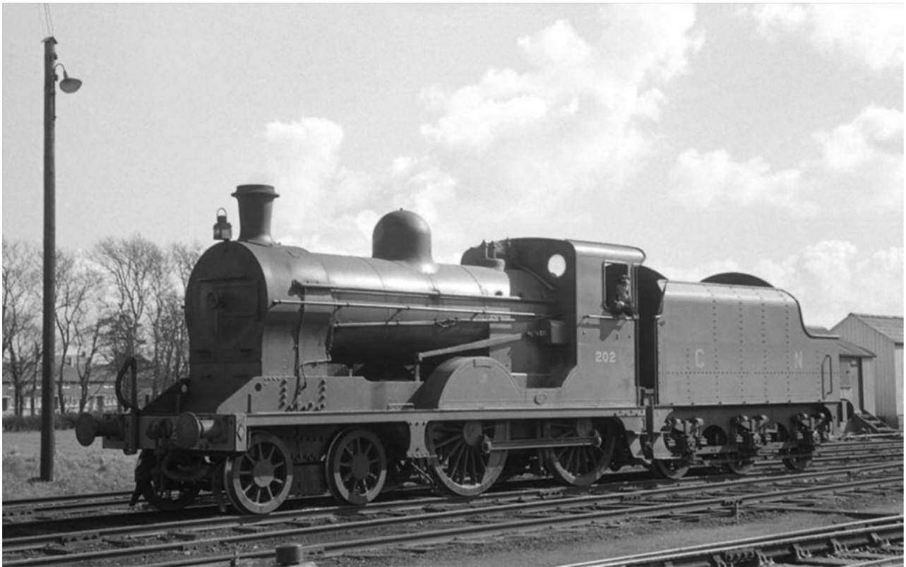
No.202 Louth at Dundalk Junction, 27 th March 1951. No.202 is of the 1948 batch, distinguished by the rectangular cab cut-out and the more modern, Stanier-esque tender design.
