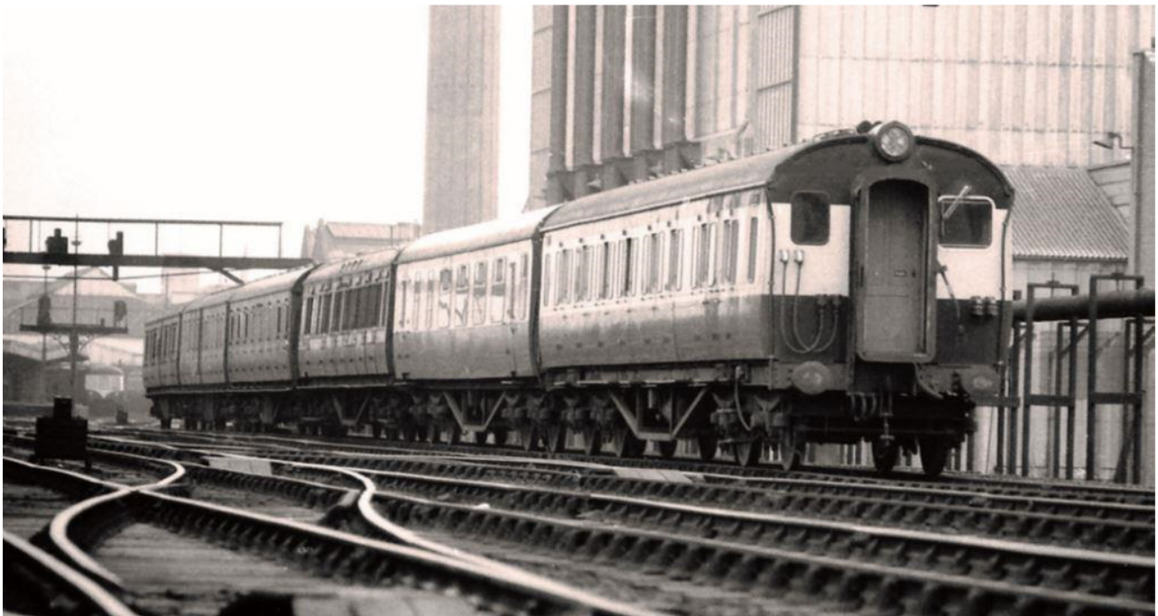
A motley collection of carriages at Belfast York Road station. Nearest the camera is a 70 class power car, followed by a purpose built 70 class trailer; the remainder are non-corridor NCC stock. An MED waits at the platform in the distance.
