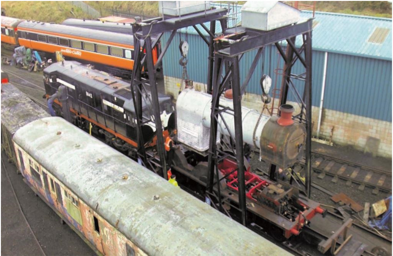
The trusty shear legs in use to fit No.131’s boiler on 21 st December 2014.
