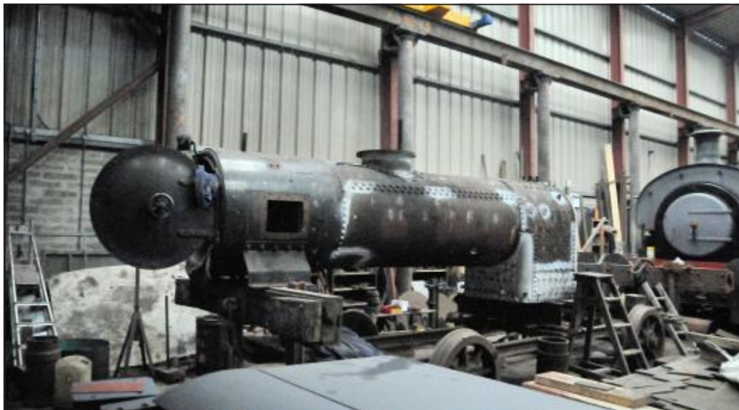
The Orenstein and Koppel boiler from Downpatrick under overhaul on 17th July 2016. Guinness 3BG, to the right, has already regained its freshly repaired boiler. The Guinness engine returned to steam on 9th October.
