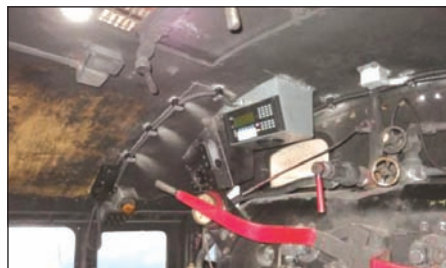
No.4's Irish Rail radio, installed spring 2017. Perhaps the point where the ability to make the electrics fit in with their surroundings was lost! (Photo: J Friel)
