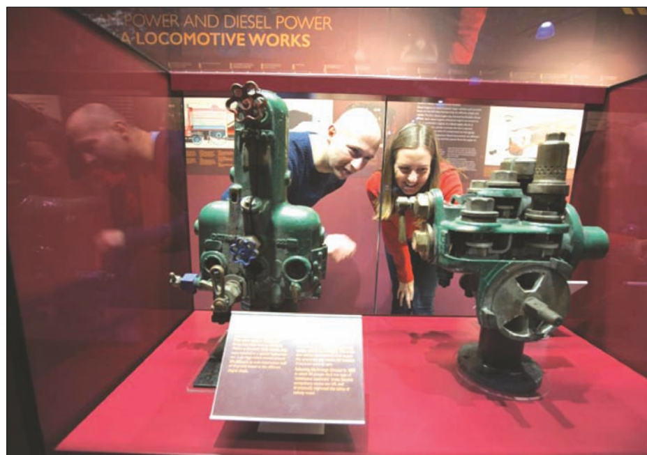
WRM visitors get a good look at many smaller artefacts that were hidden away for years, such as the sectioned hydrostatic lubricator and brake ejector once used to help train GNR(I) footplate crew. (Photo: M McCormick)
