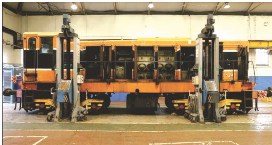
Work is well underway with the overhaul of 134 in Inchicore works. The GM 645 power unit is in good order despite its age. It will undergo a thorough inspection and have component replaced as required. The loco is on works bogies, its own having been dismantled for refurbishment. (Photo: G Mooney)
