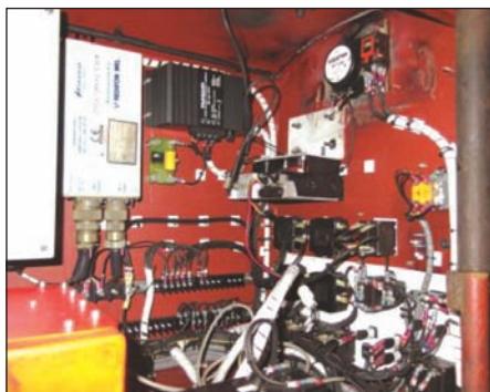
Nos.85 & 131's new brains are in replica toolboxes behind the driver. The large orange box is the OTMR. The rest permits you over 40mph! (Photo: J Friel)
