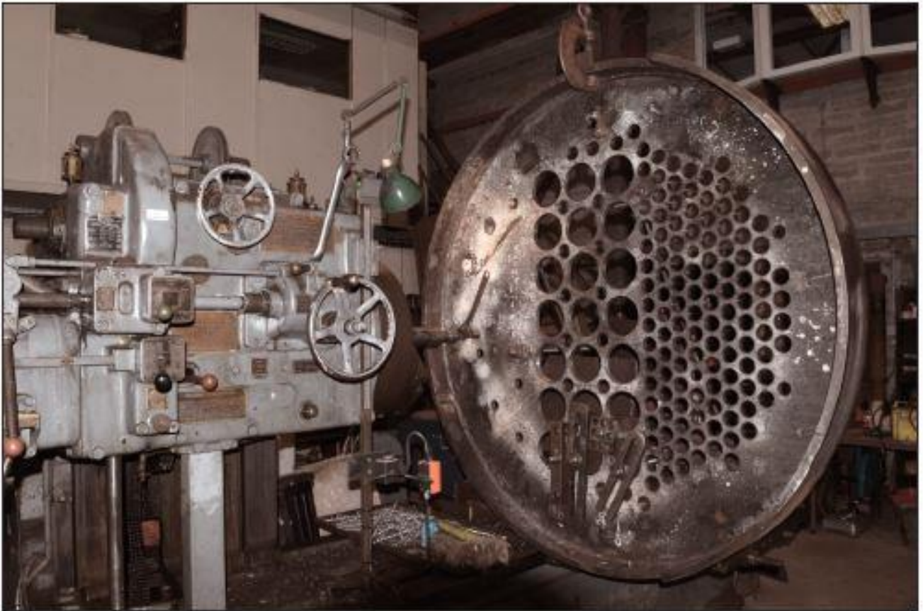
Tapping steam pipe stud holes in the smokebox tubeplate of the second NCC boiler on 27 th October. (Photo: B Hill)
