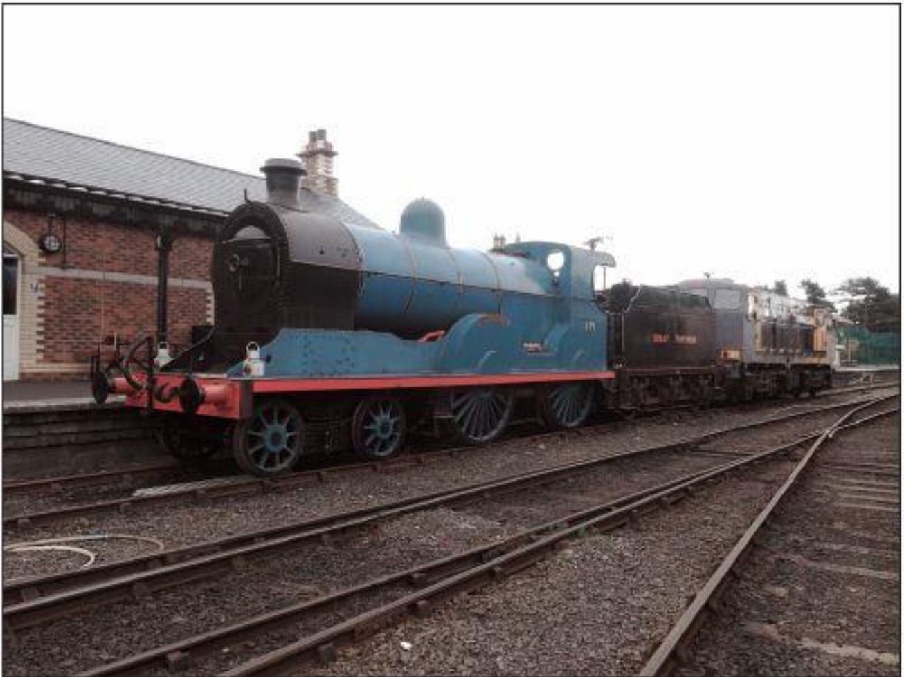
142 propels No.171, who is wearing No.131's tender, her own as yet being un-electrified, on 21 st May. Each new class of engine fitted with TPWS must go through a "First of Class" test to prove that the aerial on the locomotive, which picks up the signal aspect from a grid in the track seen under the bufferbeam, is performing correctly. (Photo: J Friel)
