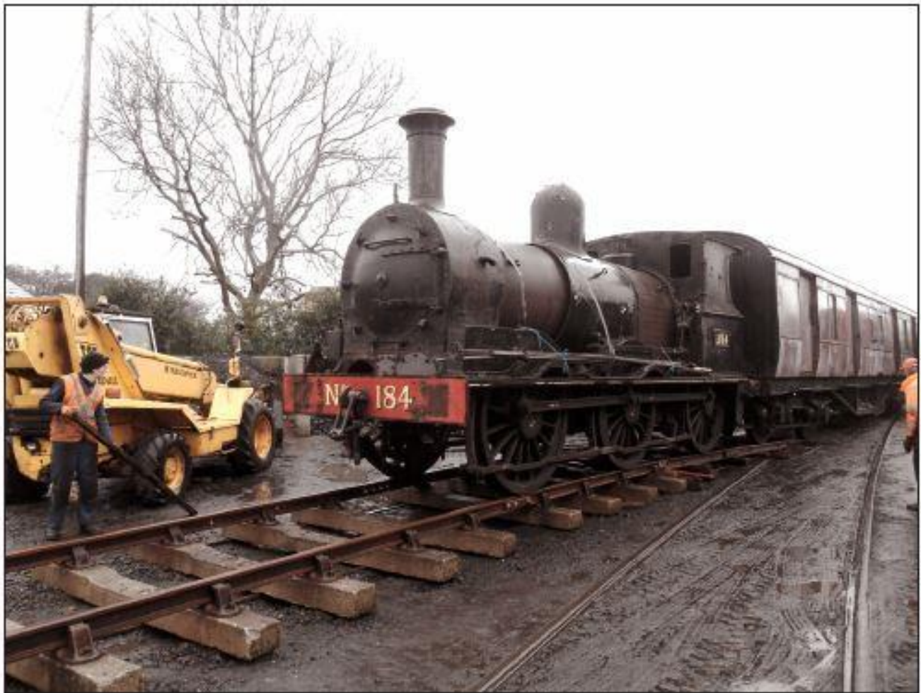
James Friel and Dermot Mackie watch on 21 st January as No.184 is cautiously pushed up onto the ramp, which is acting as a temporary bridge to take Nos.184 and 27 over the gap between the Turntable Road and the disconnected 5-Road. When both locos are on the bridge, the sloping section will be dismantled and rebuilt at the opposite end of the bridge so the engines can be moved off into the loco shed for display. (Photo: Editor)
