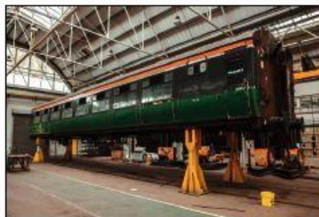
1539 in fleet casualty, Inchicore, following work to steam heating and awaiting refurbished bogies from Whitehead (Photo; S Comiskey)
