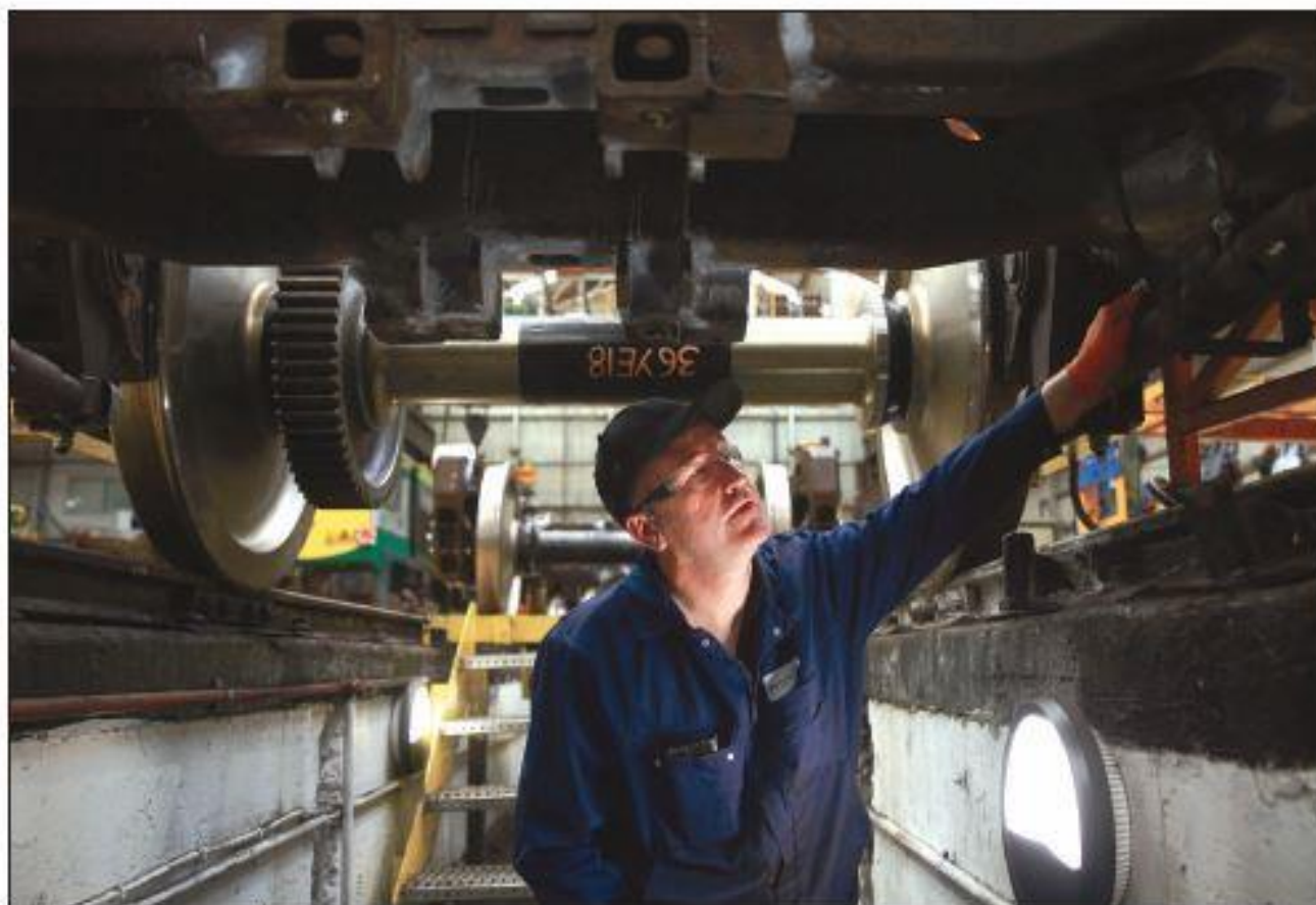
With a nice new axle, with nice new wheels and refurbished bullgear on it, above his head; Fitter Oliver Dunne checks the clearance of the newly fitted axles on bogie No2 from 134. (Photo: G Mooney)
