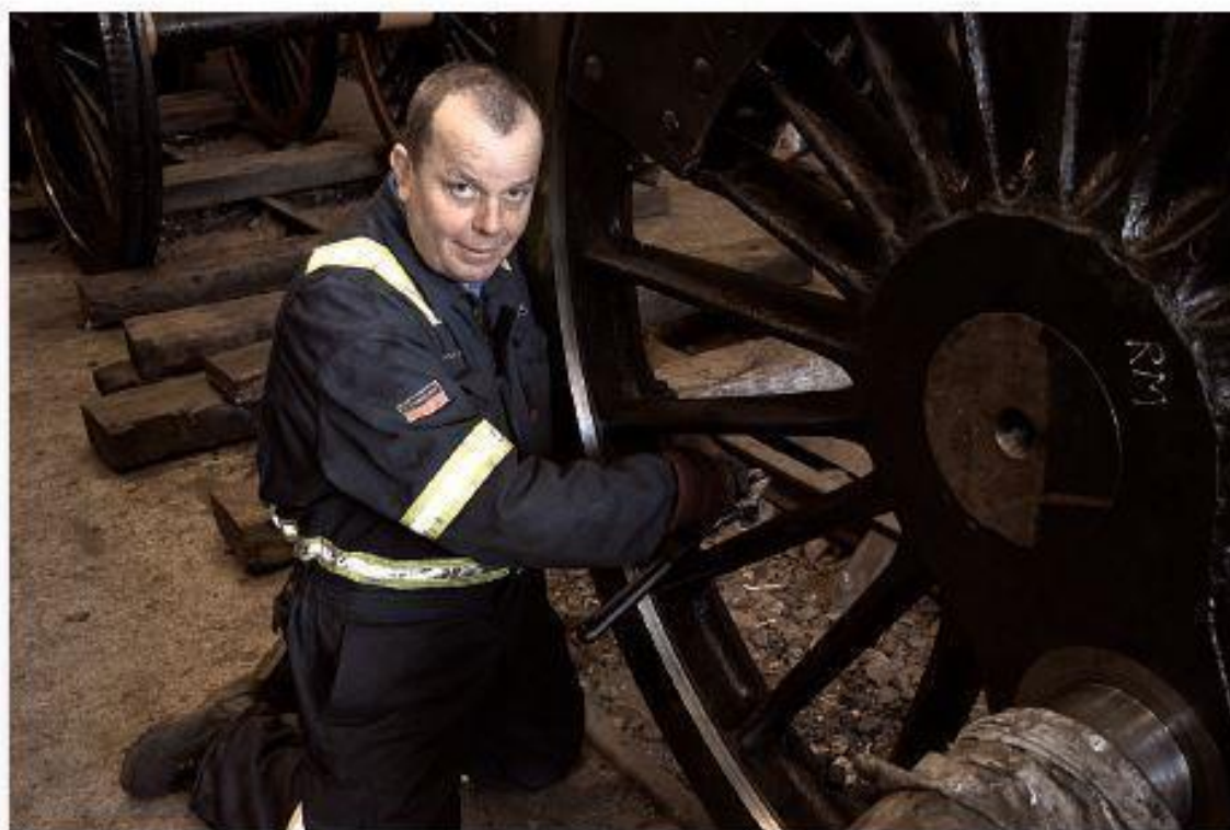
Jim Adams on 27th March fitting set screws to one of No.4's driving wheels to secure the new tyre in place. (Photo: B Hill)
