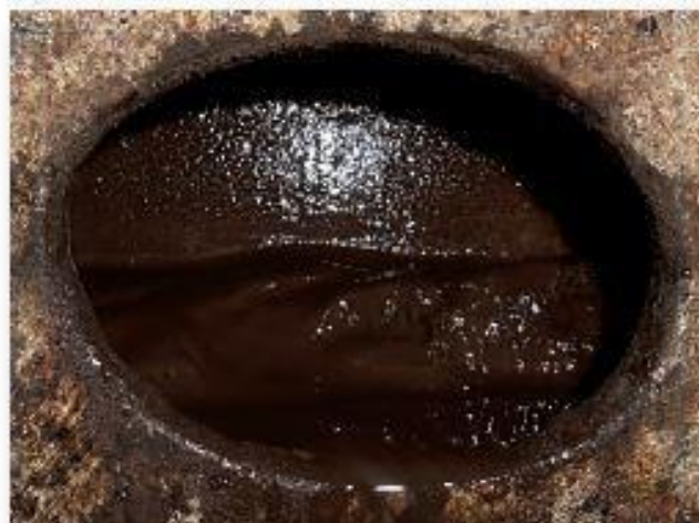
A mud-door hole with silt behind, No.4, 11th January. (Photo: Editor)
