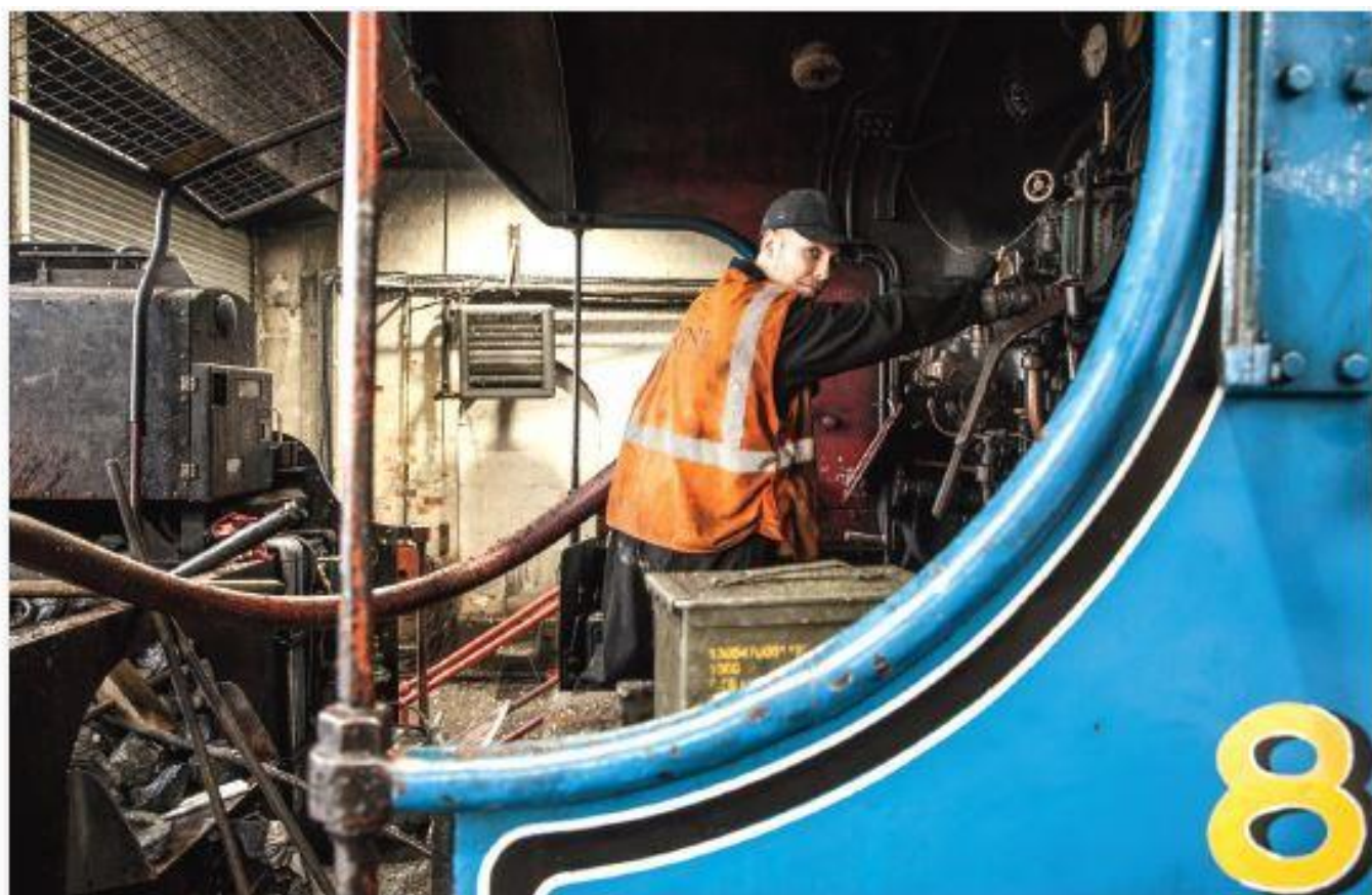
Zachary Westhelle Hartfiel inserts a firehose nozzle into a faceplate washout plug hole on No.85, Connolly Shed, 24th November. The same method is described later as now used at Whitehead. Dublin have the power and volume of the Connolly water tank pump behind them! (Photo: S Comiskey)
