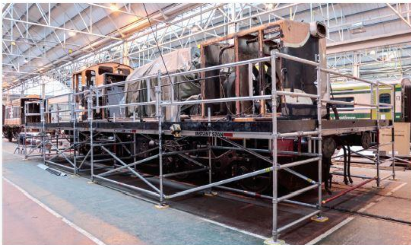
Locomotive 134 surrounded with its bespoke work platform in the lifting shop of Inchicore Works on 04th December. (Photo: G Mooney)
