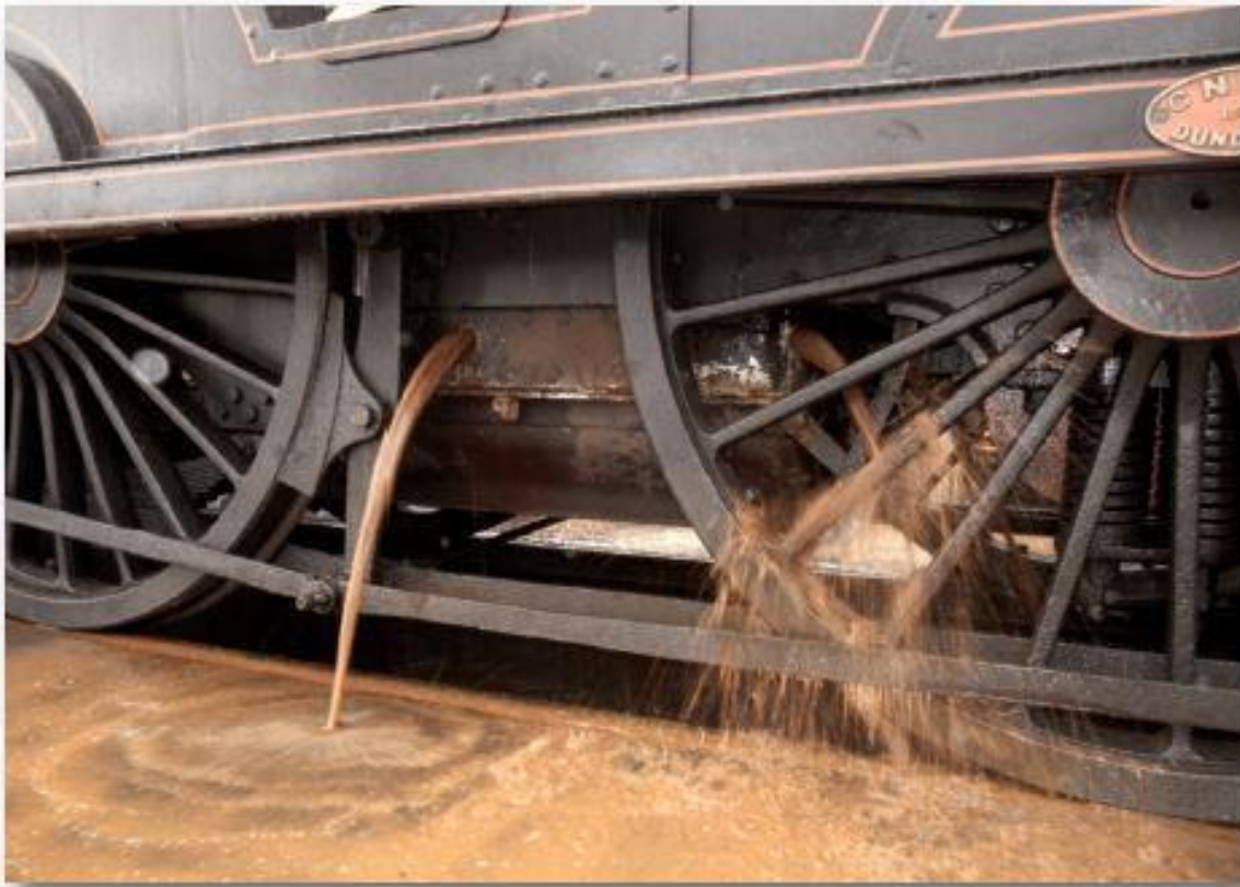
Mud and mess exit No.131 PDQ on 17th November, following connection to Whitehead's brand-new petrol-driven pump. (Photo: Editor)
