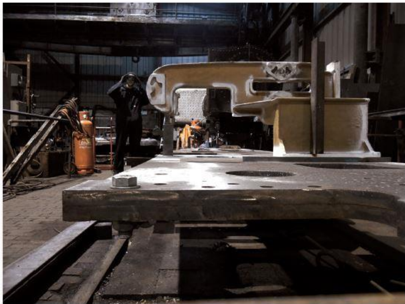
On 05th January 2020 a newly-cast (in Scotland) motion bracket sits in place on the frames of No.105. See inside cover photo of No.4 for identical motion bracket. Behind them, No.171's boiler is sideways on the rotator. Nathan Lawrence prepares to drill holes in the rear of the frames. [Photo: Editor]
