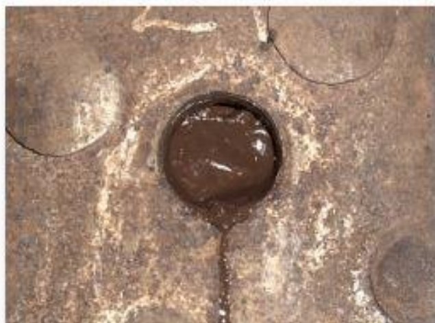
A silted-up foundation ring washout plug hole, No.4, 04th January. (Photo: Editor)
