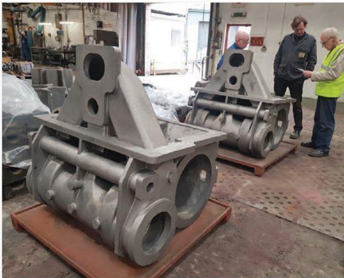
Photos such as this are normally in black and white and of places like Harland & Wolff a hundred years ago. But this is at Taylors foundry at Hamilton, Scotland on 06th August and shows Peter Scott, in yellow, with the two cylinder block castings for No.105 fettled up, blast cleaned and ready for despatch to Whitehead. Remarkable.
