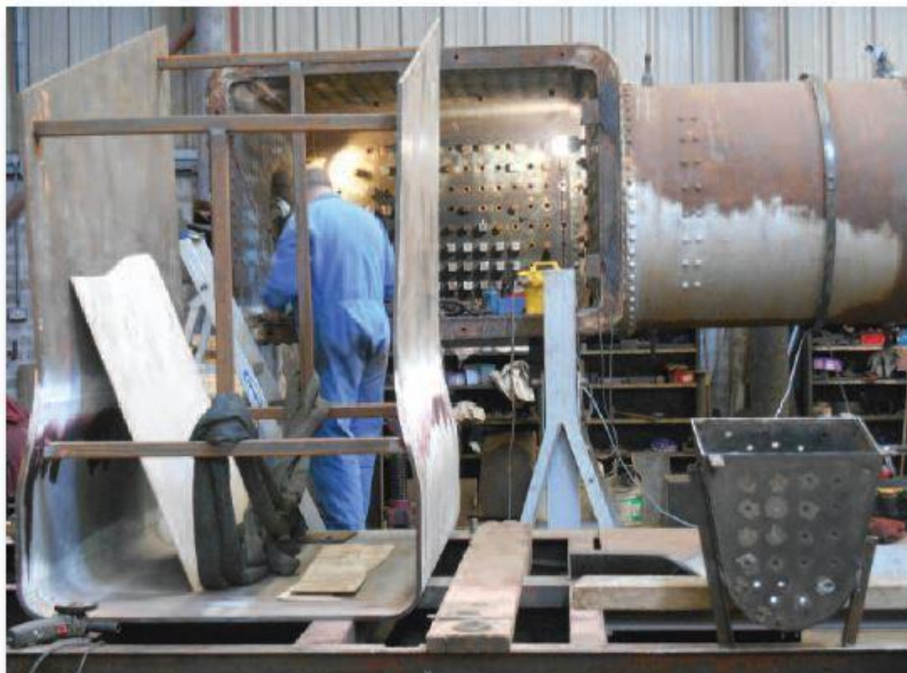
Three fireboxes in the workshop on 27th September. On the boiler rotator in the background, new crown stay bolts can be seen in the firebox crown sheet of No.171. In the foreground is no gross miscalculation, for the inner copper firebox on the left is not destined for the inverted tiny steamboat boiler on the right, but for the possible boiler for No.105. (Photo: Editor)
