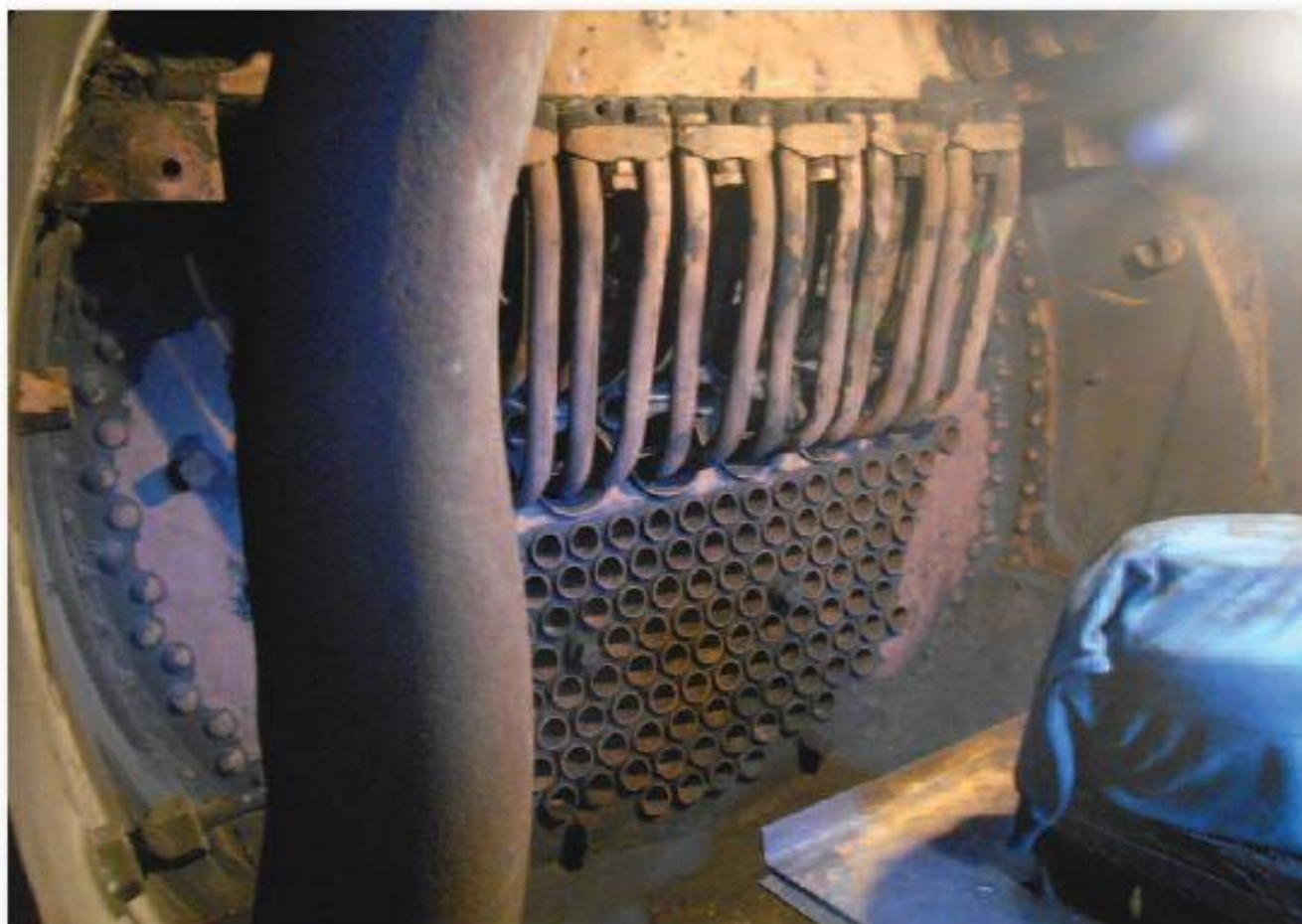
The superior, spacious smokebox of the Jeep with its self-cleaning screens removed. You even get a little seat to sit on when removing washout plugs. 'Superior' as compared to shorter, cramped GNR(1) and No.461 smokeboxes with their enormous, inevitably rusty and thorny, overall-shredding, wire-cage spark arrestors. Getting to a washout plug in these has been described as 'like getting up the beach at Normandy, except nobody is shooting at you'. They even flood for extra effect if you are not careful with your washout hose.
