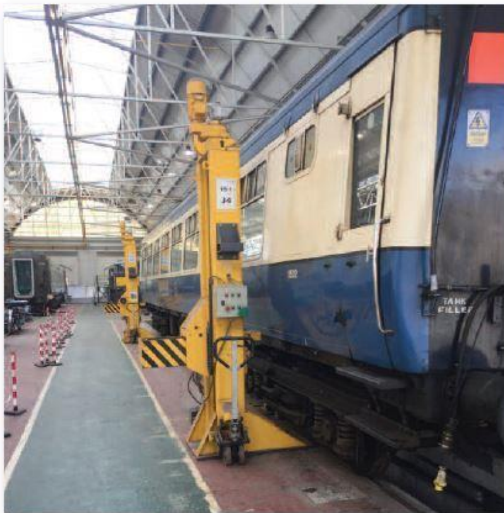
Diner 1522 in fleet casualty repair shop Inchicore on 02nd March (with some tasty jacks Whitehead would really like). The refurbished bogies will shortly be fitted. In the background is an 071 undergoing body work repairs and a MkIV coach. (Photo: P Rigney)
