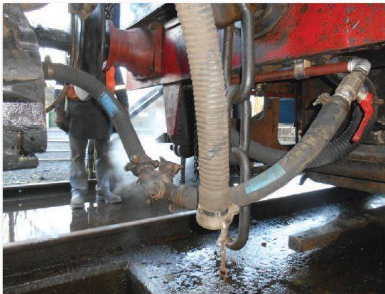
3BG's new steam heat is tested on a Mk2 on 09th February. In the foreground is the coach's veckum beg; 3BG's is behind her heat beg. (Photo: Editor)
