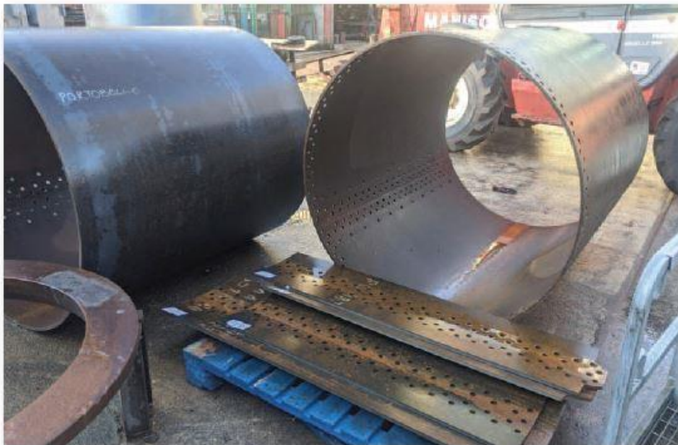
These are the newly-rolled barrel sections and joining plates (called "butt straps") for boiler G8.24, which may end up in No.105, at Israel Newton, Derbyshire, on 12th January 2021. Again, remarkable. (Photo: c/o P Scott)
