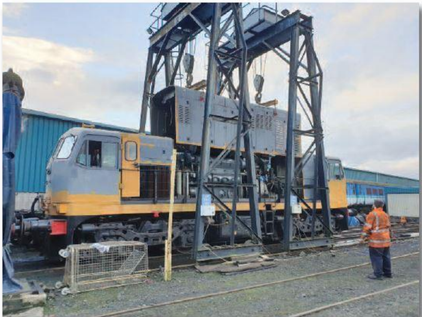
On one of the very few days post-March where it felt like a meaningfully large job was achieved in the yard on a weekend, Ryan Downey operates the sheer legs to lift B142's hood off on 19th December. (Photo: A Lohoff)
