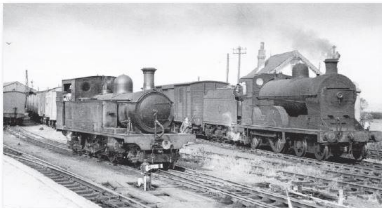
Drumboe (1958) at the north end of Strabane station alongside GNR(I) S2 Class, No 192 "Slievenamon". You can see the trans-shipment shed for traffic between the County Donegal and the GNR(I) behind "Drumboe". The Class 5 CDR tanks locos, were large superheated locomotives with a weight of over 43 tonnes. You can see a small shunting signal in the foreground and the shunter making up a goods train that includes a GNR(I) P Van, behind 4-4-0 No 192.
