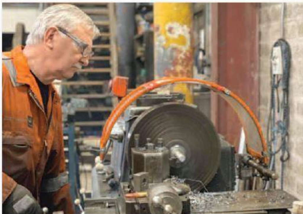
HEI's Billy Clements making crown stays for No.171, 28th October. See Page 18 for where they'll end up. (Photo: RPSI)
