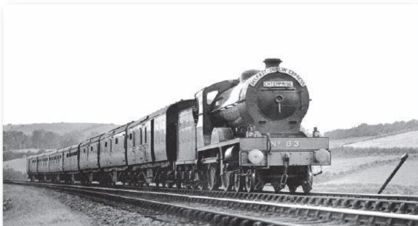
In the photograph used for the public timetable of the service, No.83, pre-Belpaire forebox, and the 7-Coach Enterprise train race through Knockarney, near Poyntzpass. (Photo: R Clements Lyttle)
