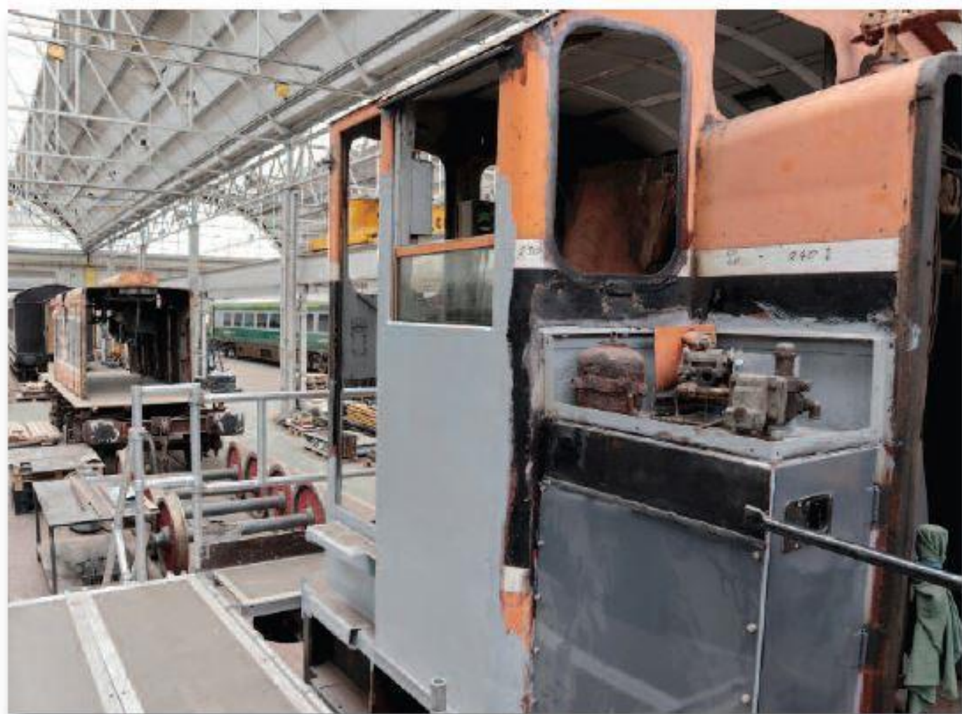
B134 Large: It's 'Taps off' for the diesels again. On 04th August, B134's bonnet sits on a wagon behind the loco, the cab of which is being refurbished. (Photo: G Mooney)
