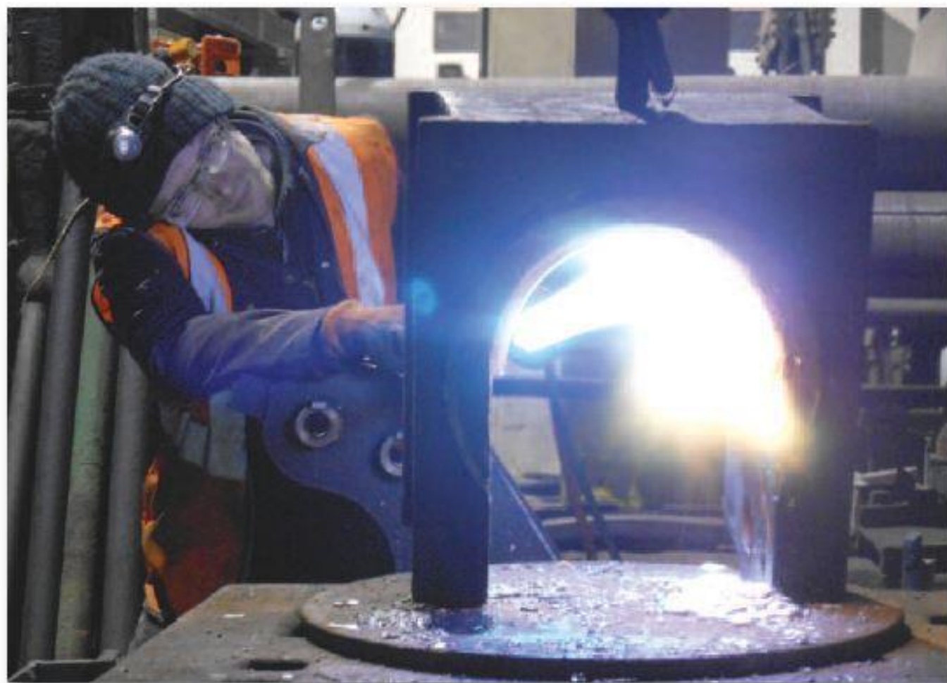
James Friel melts white metal out of a No.171 driving axlebox on 12th January.
